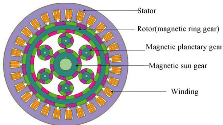
**Figure 1.** Stator hybrid excitation planetary gear motor.
