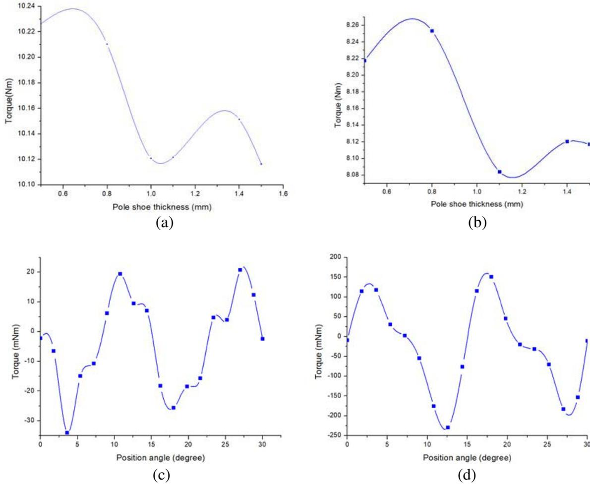
**Figure 3.** Transfer torque and positioning torque: (a) Ring gear torque; (b) Planetary ring gear torque; (c) Positioning torque characteristics of permanent magnet planetary gears; (d) Positioning torque characteristics of permanent magnet sun gear.
