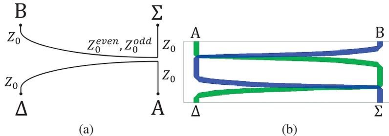
**Figure 1.** (a) Schematic of an asymmetrically coupled transmission line. (b) Offset stripline implementation of a broadside coupled transmission line hybrid. Two 8.34 dB couplers are cascaded together to realize a 3 dB,  $180^\circ$  hybrid coupler.
