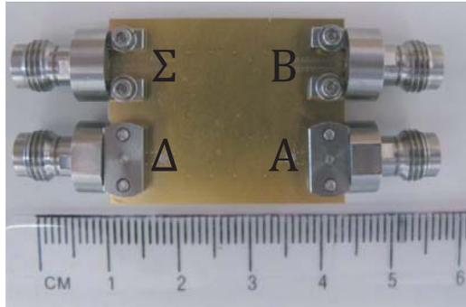
**Figure 8.** Fabricated hybrid coupler.
