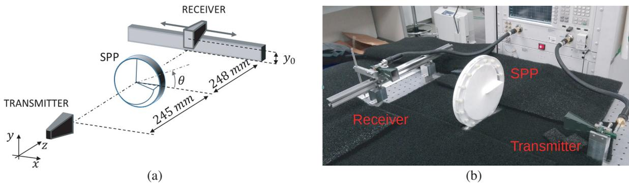
**Figure 2.** (a) Geometry of the experimental setup. The scan has been performed in the horizontal  $x$  direction through a linear translation stage positioned at two different vertical positions from the singularity. (b) Picture of the experimental setup.
