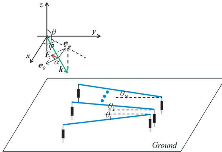
**Figure 1.** Typical model of NPTLs on the ground excited by ambient wave.
