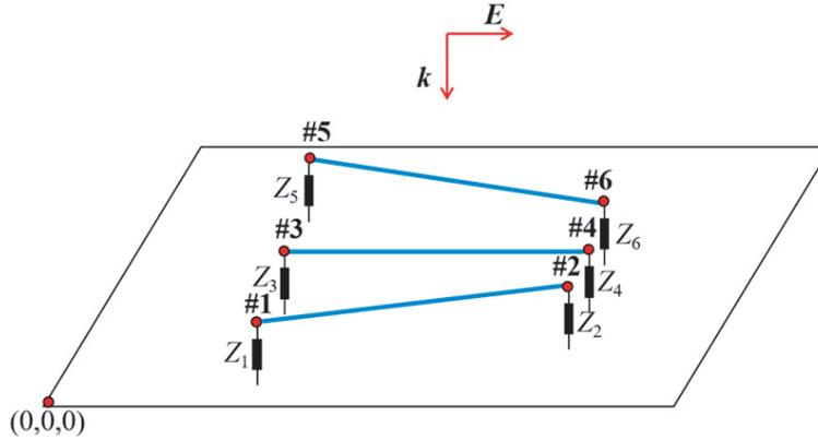
**Figure 6.** Coupling model of MTLs on the PEC ground excited by ambient wave.
