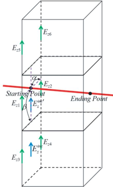
**Figure 5.** Interpolation scheme for the electric fields at starting and ending points of each segment.
