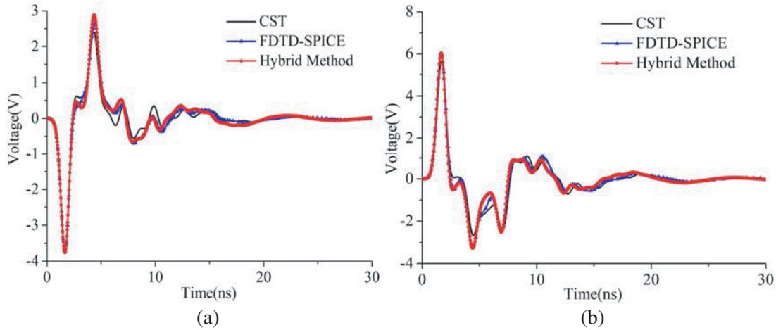
**Figure 7.** Voltage responses on the loads of NPTLs computed by the three methods for the first case. (a) Voltages on load  $Z_1$ . (b) Voltages on load  $Z_6$ .
