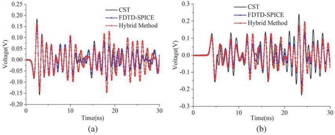
**Figure 10.** Voltage responses on the loads of NPTLs computed by the three methods for the second case. (a) Voltages on load  $Z_1$ . (b) Voltages on load  $Z_6$ .
