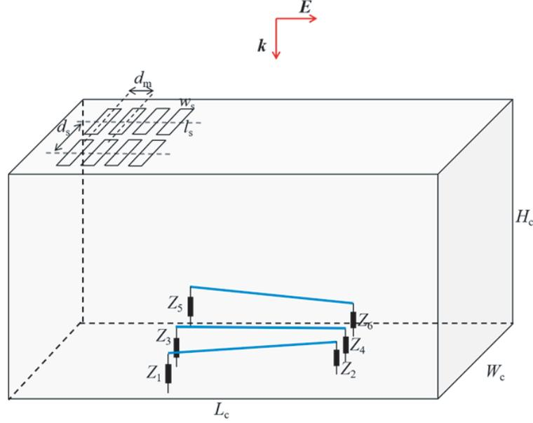
**Figure 9.** Coupling model of NPTLs in the shielded cavity.
