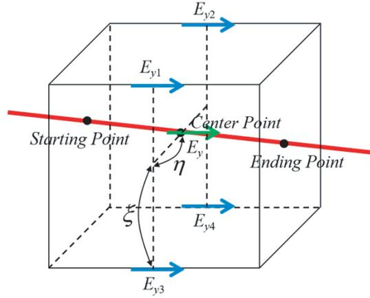
**Figure 4.** Interpolation scheme for the electric fields at the center point of each segment.
