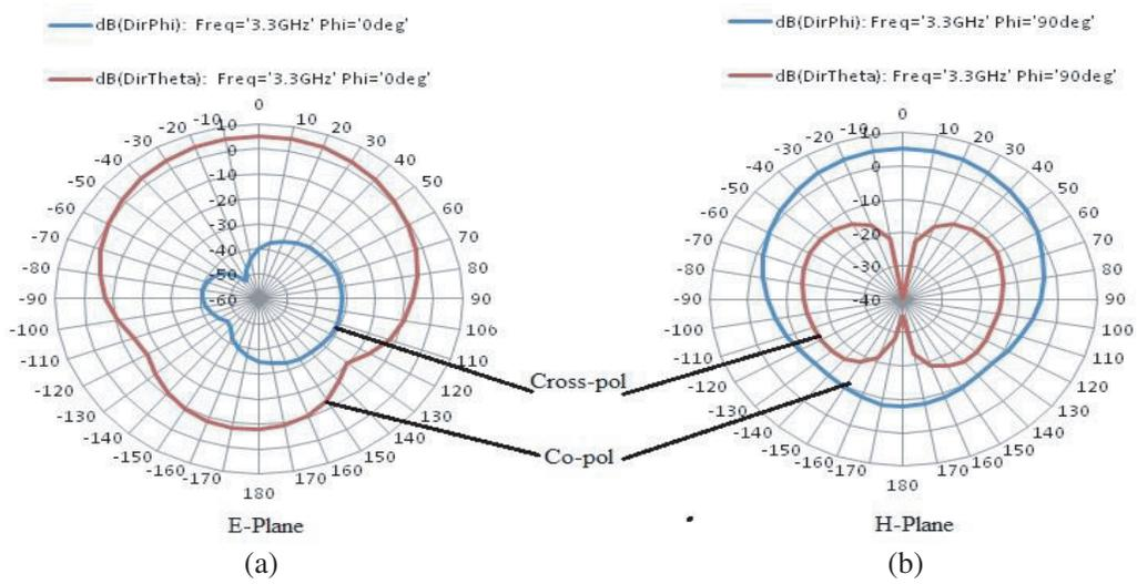
Figure 9. Cross polarization effect at lower frequency band (a)  $\phi = 0^\circ$ . (b)  $\phi = 90^\circ$ .
