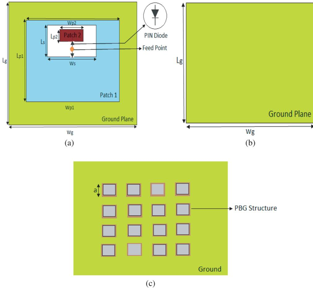
**Figure 1.** Geometry of the proposed antenna. (a) Top view. (b) Bottom view without PBG. (c) Bottom view with PBG.
