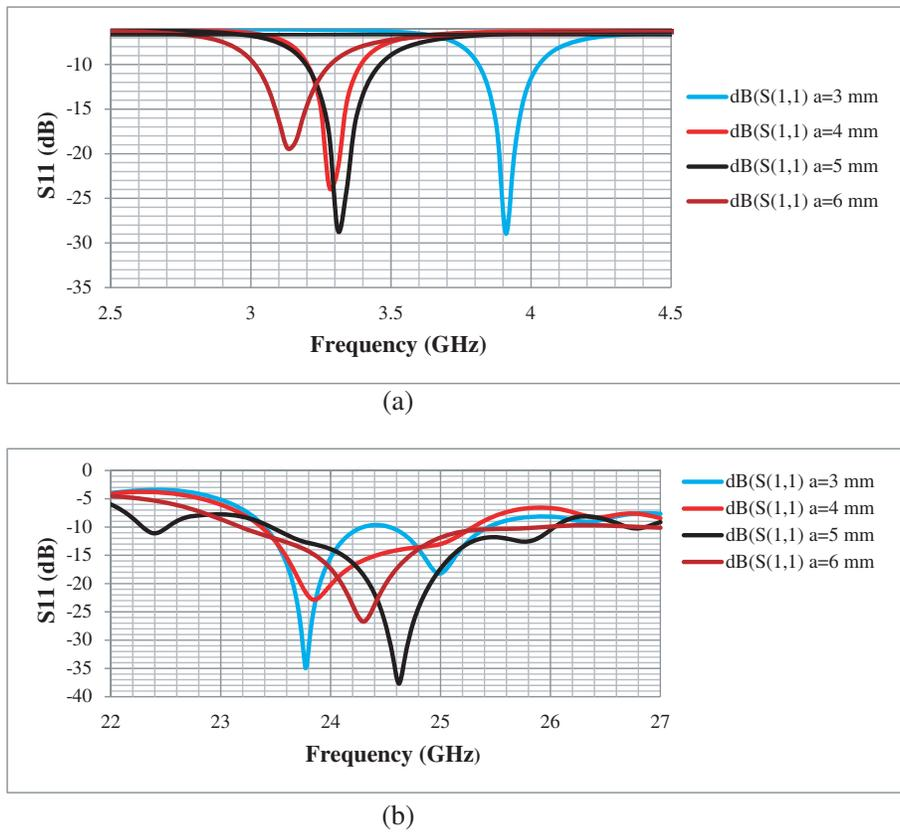
Figure 5. Return loss at different PBG dimensions for (a) lower band, (b) upper band.
