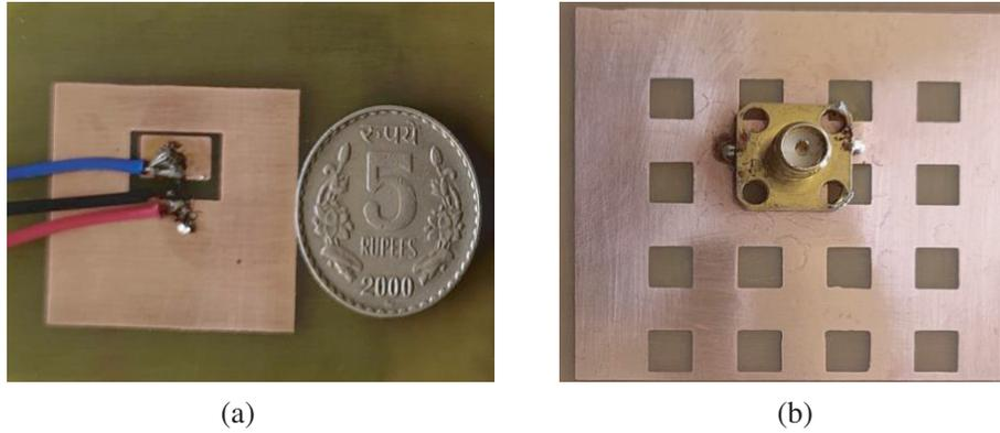
**Figure 2.** Fabricated antenna with PBG structure. (a) Top view. (b) Bottom view.
