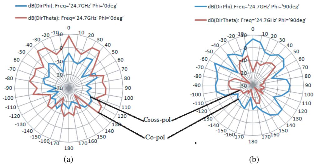
Figure 10. Cross polarization effect at upper frequency band (a)  $\phi = 0^\circ$ . (b)  $\phi = 90^\circ$ .
