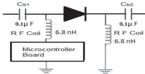
**Figure 3.** Biasing circuit using microcontroller board.
