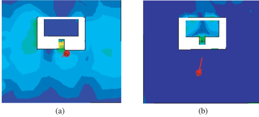
Figure 8. Surface current distribution when (a) patch 1 is excited (b), patch 2 is excited.
