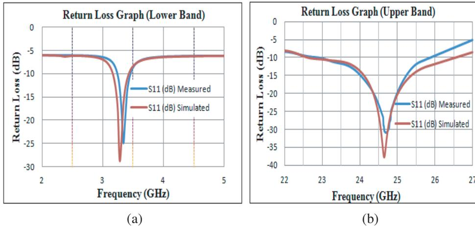
**Figure 7.** Simulated and measured return loss with PBG structure. (a) Lower band. (b) Upper band.
