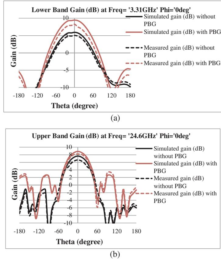
**Figure 6.** Measured and simulated antenna gain without and with PBG structure of (a) lower band, (b) upper band.
