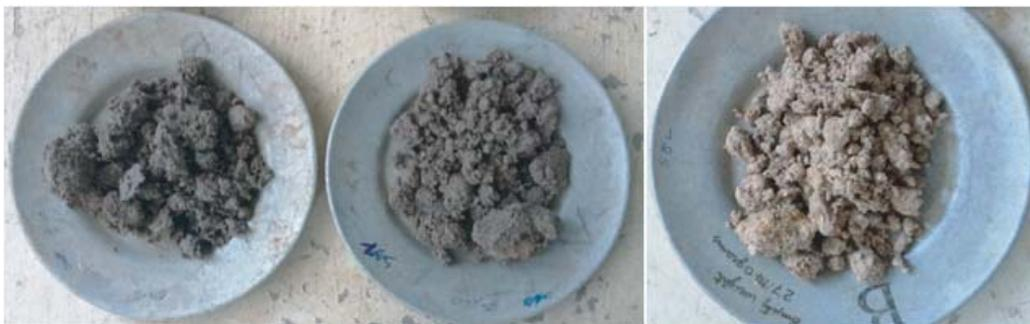
**Figure 2.** Oven dried soil samples.
