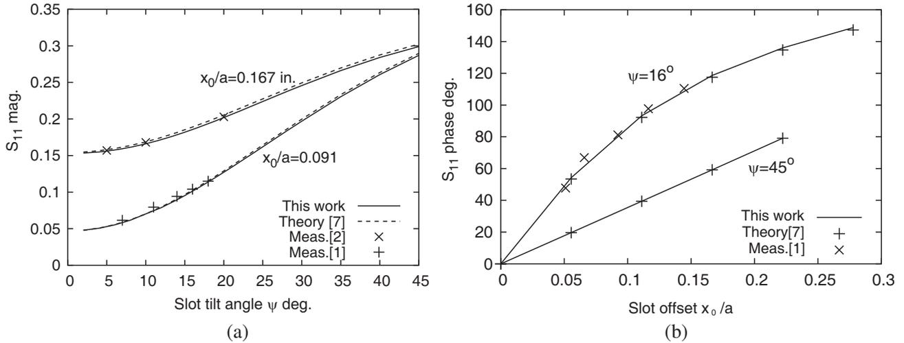
**Figure 5.** Comparison of magnitude and phase of backscattered wave at resonance with modified analytical theory [7] and measurement. (a) Magnitude of backscattered wave at resonance with tilt angle. (b) Phase of backscattered wave at resonance with tilt angle.
