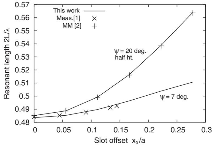
**Figure 4.** Resonant length with slot offset compared with measured [1] and mode method (MM) results [2].
