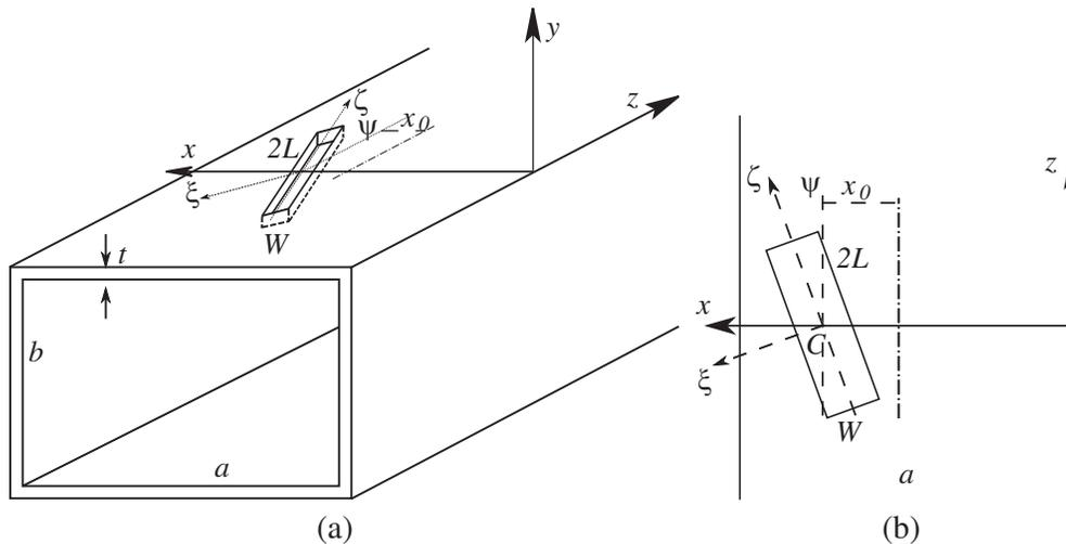
**Figure 1.** Geometry of the problem. (a) Waveguide fed compound slot. (b) Top view of the waveguide with compound slot.
