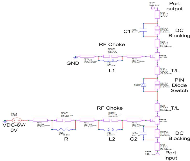
**Figure 7.** Schematic representation of the switching circuit components inserted in active feeding network.
