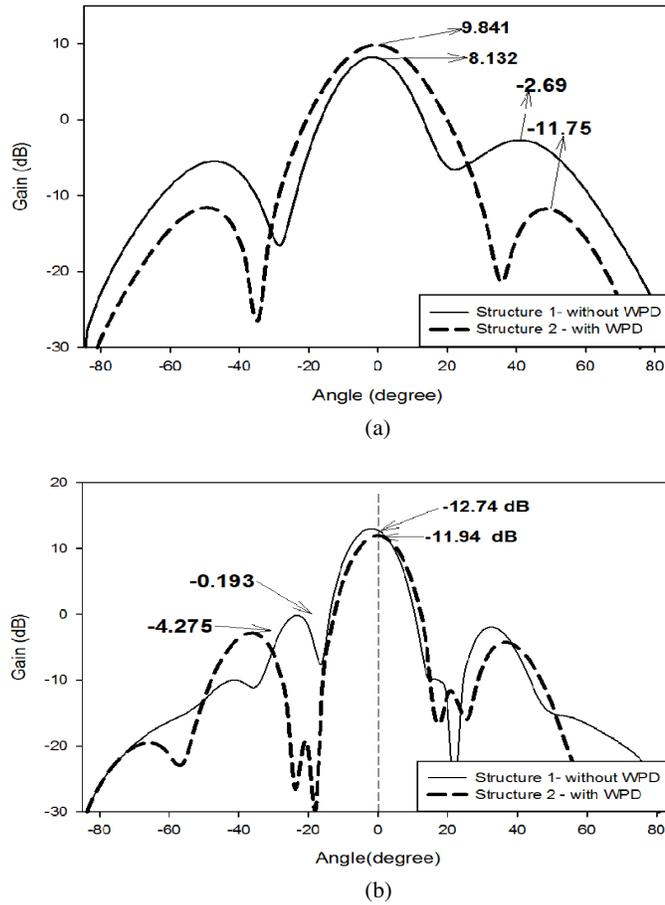
**Figure 6.** Comparison of radiation pattern between antenna structure 1 and 2 (a) 4 radiated elements (b) 8 radiated elements.
