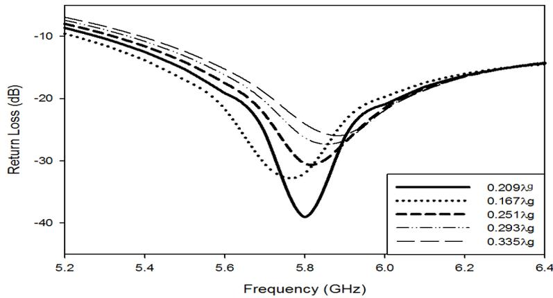
**Figure 2.** Return loss due to length of 100 Ω transmission line.
