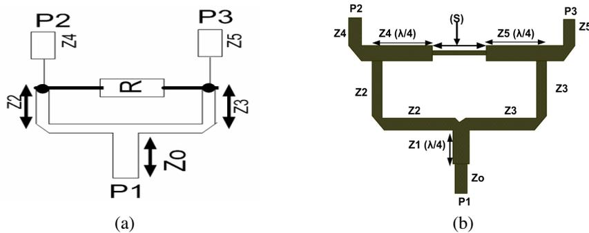
**Figure 1.** (a) Conventional Wilkinson power divider (b) the modified Wilkinson power divider geometry.
