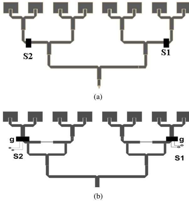
Figure 4. Configuration of two structures of corporate fed reconfigurable antenna array (a) Structure 1 (without WPD) (b) Structure 2 (with modified WPD).
