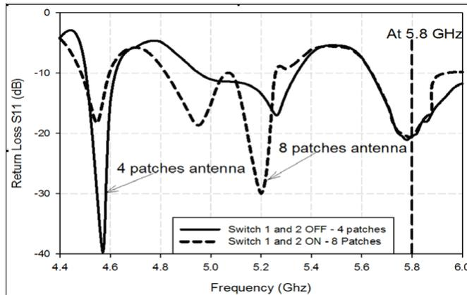
**Figure 11.** Measured results of  $S_{11}$  when switch on/off state.
