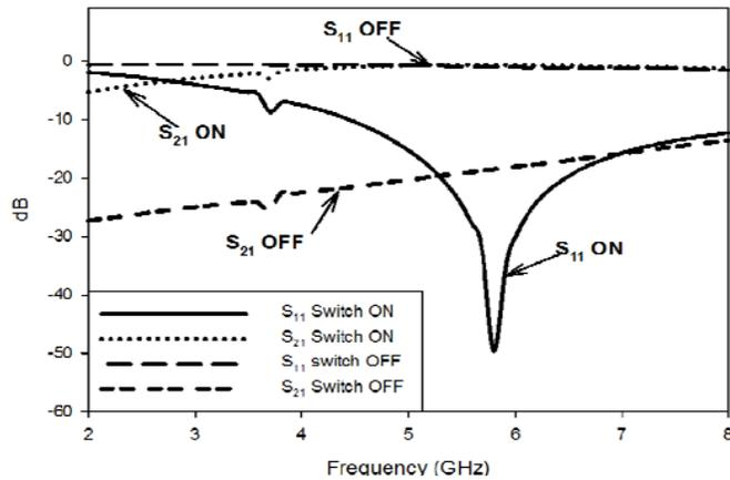
**Figure 8.** Calculated return loss ( $S_{11}$ ) for ON and OFF states (a) switch ON mode and (b) switch OFF mode.
