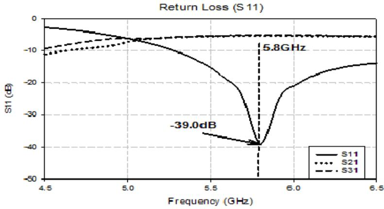
Figure 3. Return loss plot for modified WPD.
