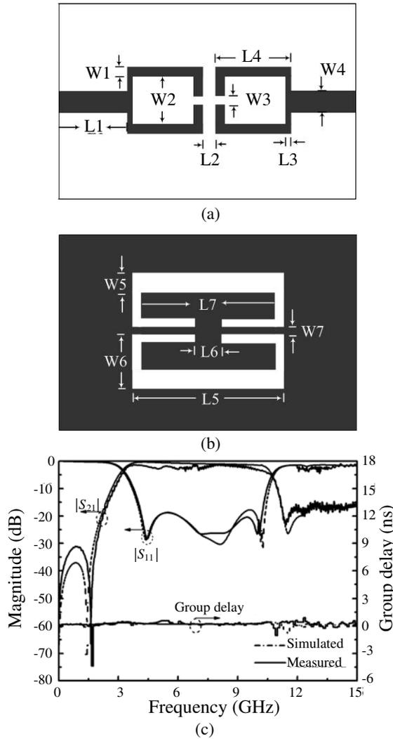
**Figure 2.** (a) Schematic top view of ultra-wideband filter. (b) Schematic bottom view of ultra-wideband filter. (c) Simulated and measured results of ultra-wideband filter.
