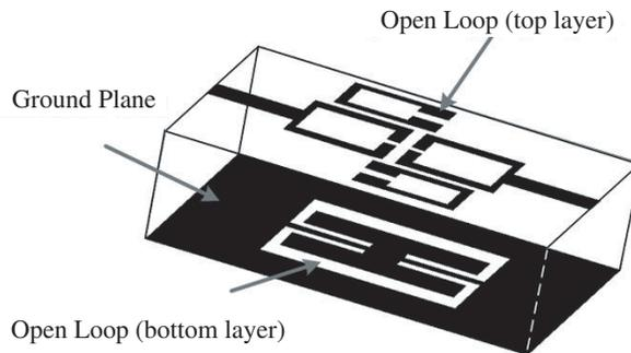
**Figure 1.** Proposed UWB filter with notch band.
