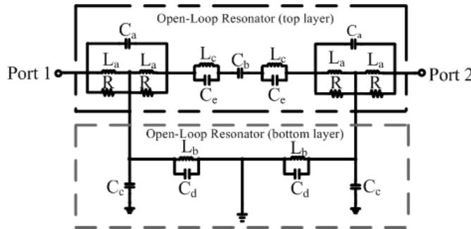
**Figure 5.** Equivalent circuit of UWB with notch band.
