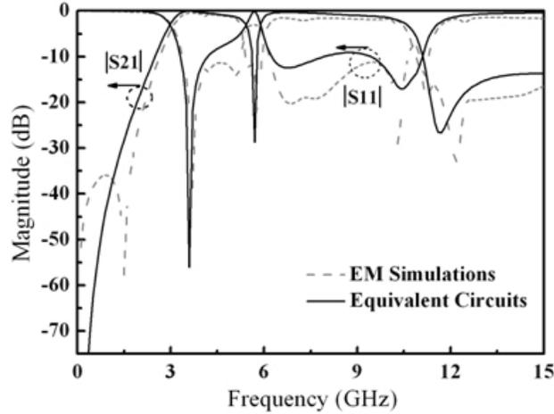
**Figure 6.** Circuit model simulation and EM simulation results.
