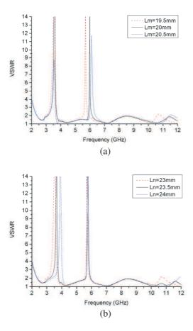
**Figure 4.** (a) Simulated VSWR for the proposed antenna in terms of  $L_m$  ( $L_n = 23 \text{ mm}$ ); (b) simulated VSWR for the proposed antenna in terms of  $L_n$  ( $L_m = 19.5 \text{ mm}$ ).
