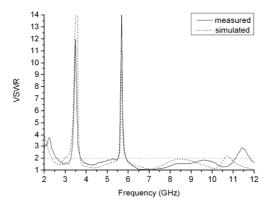
Figure 2. The comparision of the measured and simulated VSWR results.
