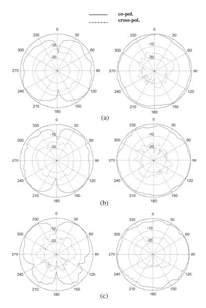
Figure 5. Measured E plane (left) and H plane (right) radiation pattern of the proposed antenna (-10 dB/div) at (a) 3.1 GHz, (b) 4.5 GHz, (c) 7.5 GHz.
