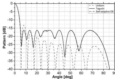
**Figure 12.** Optimum array pattern for the phase-optimized 20 elements LA, compared with uniform array.
