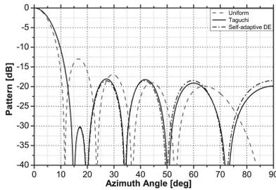
**Figure 10.** Radiation pattern of the 10 elements LA optimized with respect to positions (close-in SLL suppression case).
