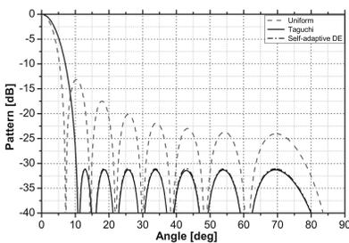
**Figure 4.** Radiation pattern of 16 elements  $\lambda/2$  spaced array optimized with respect to amplitudes, compared with uniform array.
