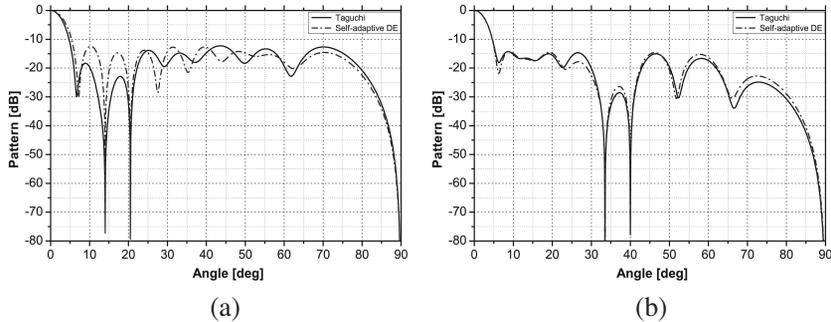
**Figure 15.** Optimum array patterns of 20 element array by the phase-only synthesis with bidirectional null steering. (a) Null steering at 14 and 20.5 degrees. (b) Null steering at 33.5 and 40 degrees.
