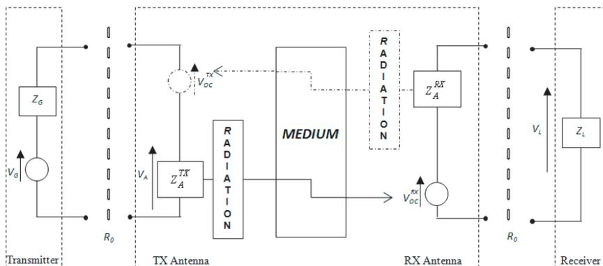
**Figure 6.** Electric model of the transmission taking into account the mutual coupling.
