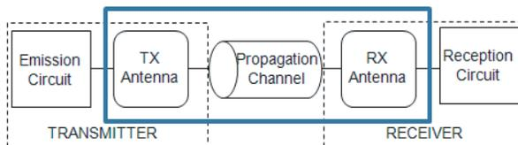
**Figure 1.** Block diagram of wireless communication system.
