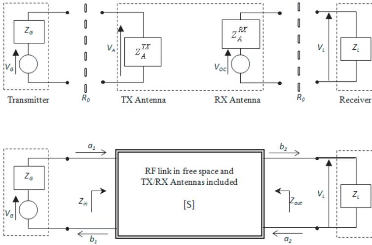
**Figure 5.** Modeling of the transmission: equivalent circuit model and  $S$ -parameters model.
