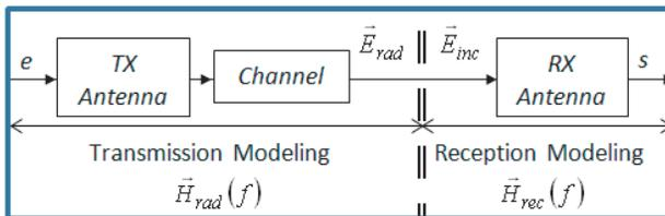
Figure 2. Block description of the modeling of the radio link.
