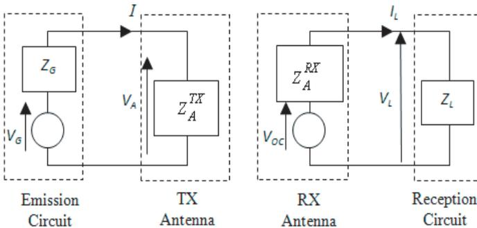
**Figure 4.** Modeling from equivalent electric circuits.
