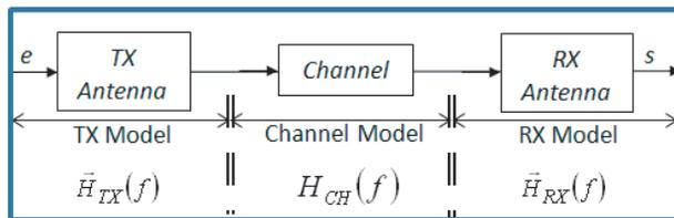
Figure 3. Radio link modeled from three functional blocks.
