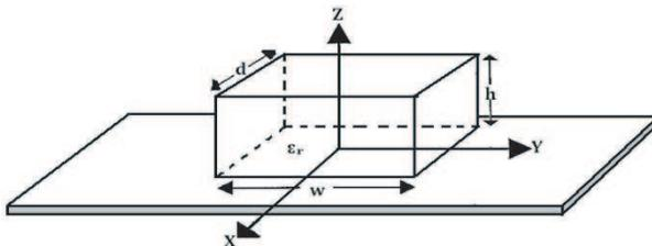
**Figure 1.** Geometry of RDRAs on finite ground plane.
