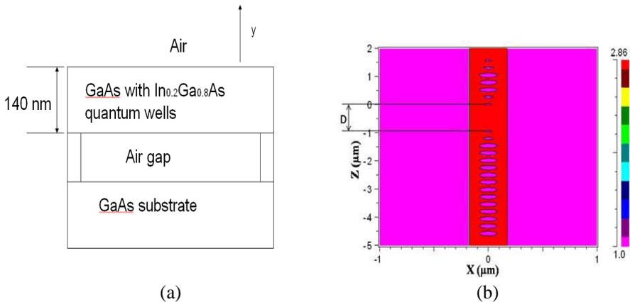
**Figure 1.** (a) Epitaxially layered structure of the photonic wire lasers. (b) Top view of a photonic wire laser.
