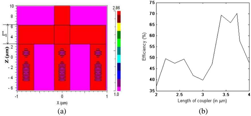
**Figure 3.** (a) Multimode interference coupler used to combine the power coming from three different photonic wire sources. (b) Coupling efficiency as a function of the length of the coupler.
