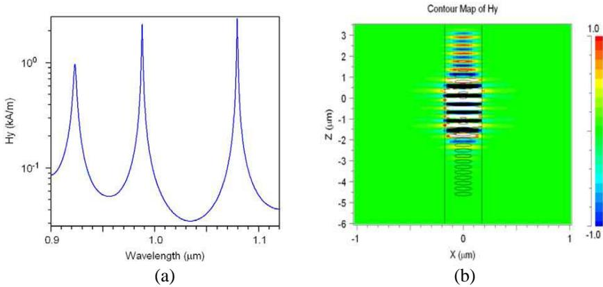
**Figure 2.** Basic photonic wire laser: (a) Magnetic field spectrum ( $H_y$ ) at the center of the waveguide. (b) Magnetic field ( $H_y$ ) distribution at  $\lambda = 987.82 \text{ nm}$ .
