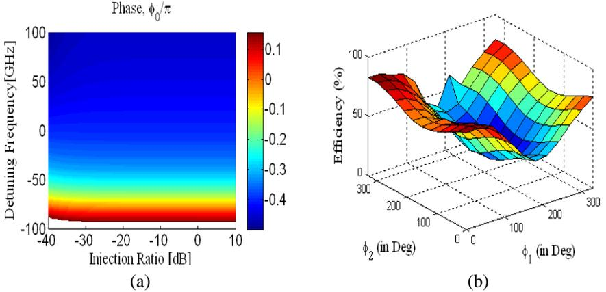
**Figure 7.** (a) The contour map showing the phase difference between master and slave laser for different values of injection ratio and detuning frequency. (b) Coupling efficiency as a function of the difference in phase from the middle laser to the lasers at the right and left.
