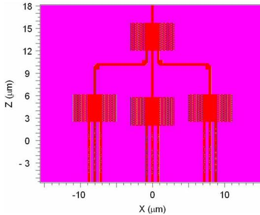
**Figure 6.** Array of 9 laser coupled by four multimode interference coupler with triangular array of holes to couple the resulting field to a single mode waveguide.
