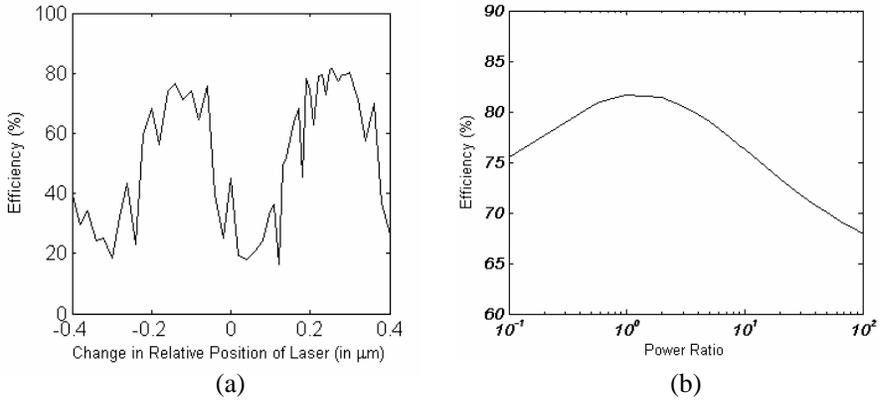
**Figure 5.** Multimode interference coupler with triangular array of holes: (a) Coupling efficiency as a function of the relative position among the sources of lasers and (b) coupling efficiency as a function of the relative power between the lasers for the optimized combiner.
