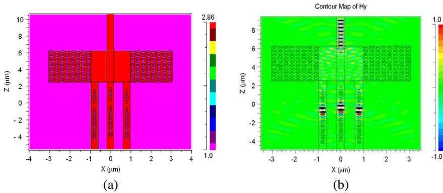
**Figure 4.** (a) Triangular array of holes added to multimode interference coupler to improve the total power in the single mode waveguide. (b) Magnetic field ( $H_y$ ) distribution at  $\lambda = 987.82$  nm for the optimized combiner.
