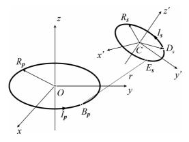
Figure 1. Filamentary circular coils with angular and lateral misalignment.
