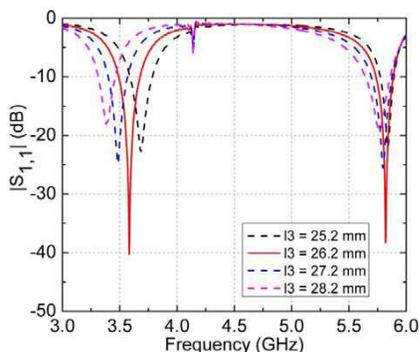
**Figure 6.** Effect of varying  $l_3$  on the return loss.
