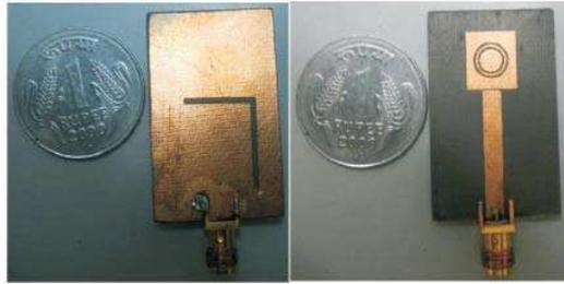
**Figure 9.** The fabricated antenna for dual band (WIMAX/WLAN) applications.
