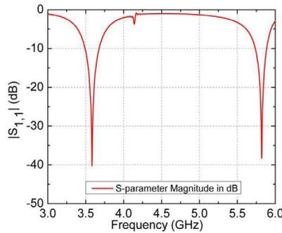
**Figure 2.** The simulated reflection coefficient of the antenna.
