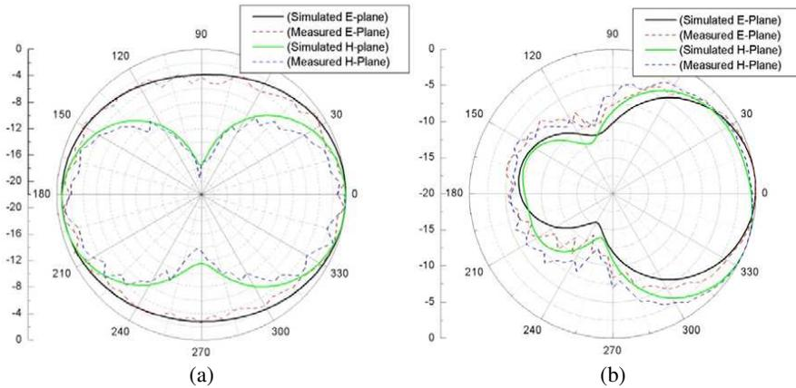
**Figure 11.** Simulated and measured  $E$ -plane and  $H$ -plane radiation pattern at (a) 3.5 GHz, (b) 5.8 GHz.
