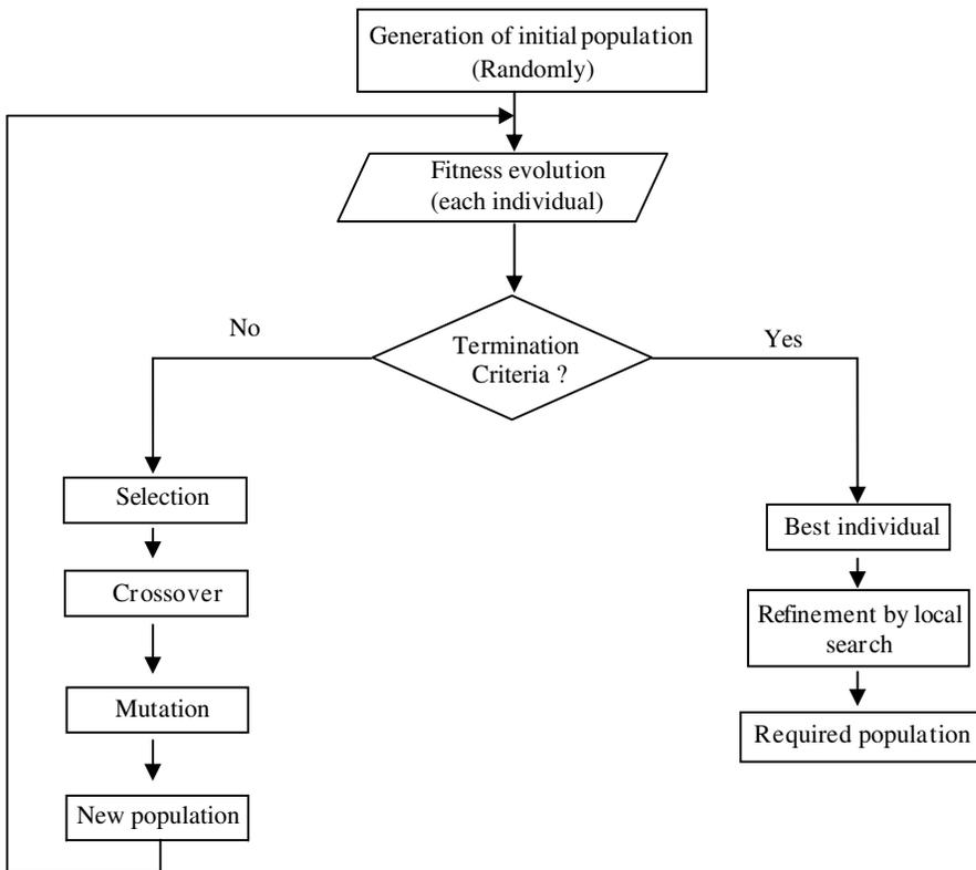
**Figure 2.** Generic flow diagram for intelligent hybrid computing.
