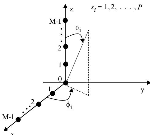
**Figure 1.** L-type array having two uniform linear arrays.
