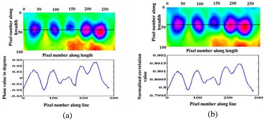
**Figure 4.** (a) Experimentally obtained phase image obtained at 0.012 Hz. (b) Experimentally obtained correlation image obtained at 20.8 s.
