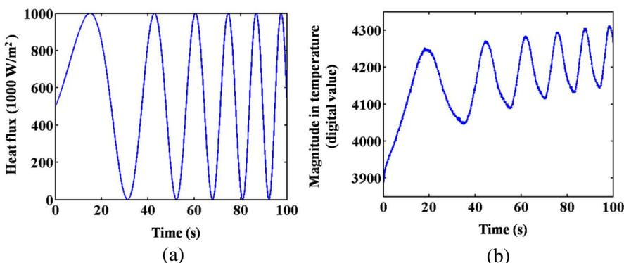
Figure 3. (a) Experimental signal used for FMTWI. (b) Temperature response over the sample during the experimentation.
