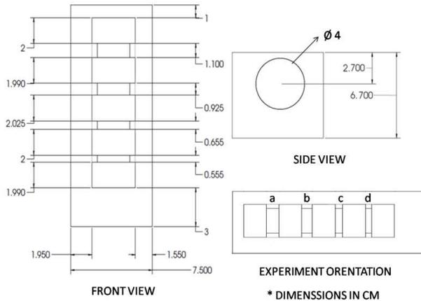
**Figure 1.** Layout of the experimental concrete sample with 40 mm mild steel rebar with groves of different widths located at same depth from the sample surface.
