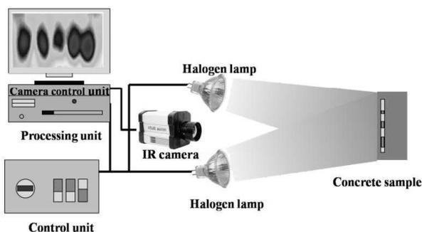
Figure 2. Experimental setup for FMTWI.
