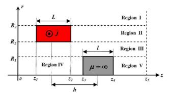
**Figure 1.** Axisymmetric system: a circular coil of rectangular cross section with an iron cylinder of finite length placed on the same axis at a distance h.
