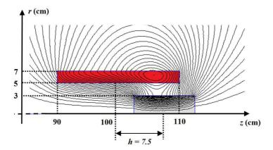
**Figure 3.** Equipotential lines around the coil for  $h=7.5\,\mathrm{cm}$  (maximum force).
