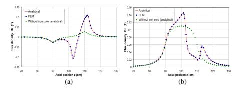
**Figure 4.** Radial (a) and axial (b) components of the flux density in Region III for  $r=4\,\mathrm{cm}$  and  $h=7.5\,\mathrm{cm}$ .
