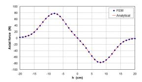
Figure 5. Electromagnetic force versus iron-core position h.
