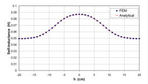
**Figure 6.** Self-inductance versus iron-core position h.
