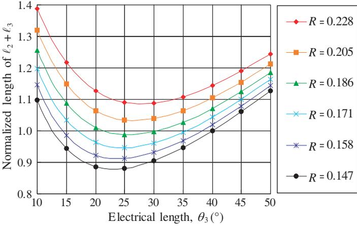
**Figure 3.** Ratio of  $Z_3/Z_2$  varies with the normalized length  $\ell_2 + \ell_3$ , to determine the electrical length of the microstrip line  $\ell_3, \theta_3$ . Length of  $\ell_2 + \ell_3$  is normalized to half of  $\ell_1$ .  $R$  is the ratio of  $Z_3/Z_2$ .
