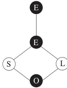
**Figure 5.** Coupling scheme of the third order passband filter.  $S$  is the source and  $L$  is the load.  $E$  is the even mode resonant frequency.  $O$  is the odd mode resonant frequency.
