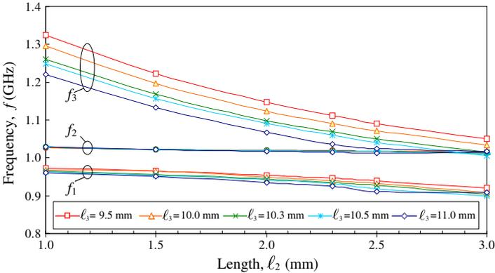
**Figure 4.** Resonant frequencies of the triple-mode resonator by varying  $\ell_2$  and  $\ell_3$ .  $\ell_2$  and  $\ell_3$  are with the characteristic impedance of  $70.44\ \Omega$  and  $11.20\ \Omega$ , respectively.  $\ell_1$  is  $29.00\ \text{mm}$ .
