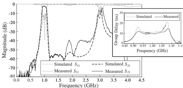
**Figure 10.** Broadband simulated results and measured results of the sixth order bandpass filter. Inset is the group delay for the first passband.
