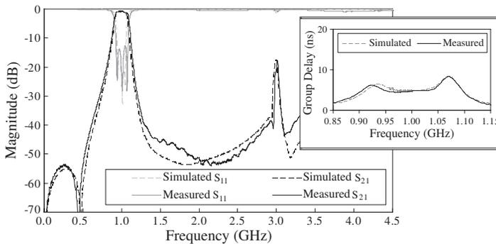
**Figure 7.** Broadband simulated results and measured results of the third order bandpass filter. Inset is the group delay for the first passband.
