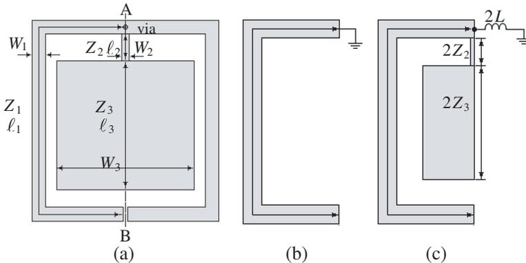
**Figure 1.** (a) Compact triple mode ring-like resonator.  $AB$  is the plane of symmetry. Equivalent circuit of the proposed triple-mode resonator: (b) odd mode and (c) even mode.
