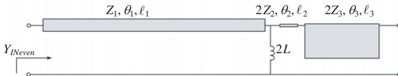
**Figure 2.** Even mode equivalent circuit of the triple-mode resonator.
