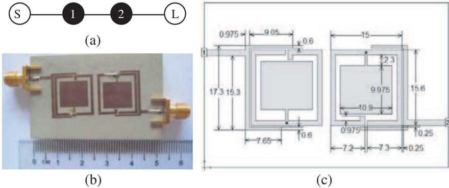
**Figure 9.** (a) Coupling scheme of the sixth order bandpass filter. Solid circle is the triple-mode resonator. The coupling of each triple-mode resonator is shown in Figure 5.  $S$  is the source and  $L$  is the load. (b) Photograph of the fabricated filter. (c) Layout of the sixth order bandpass filter designed using the proposed resonators (dimension in millimeters).
