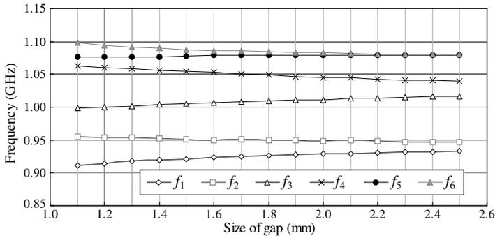
**Figure 8.** Resonant frequencies of the two coupling triple-mode resonators against the size of gap.
