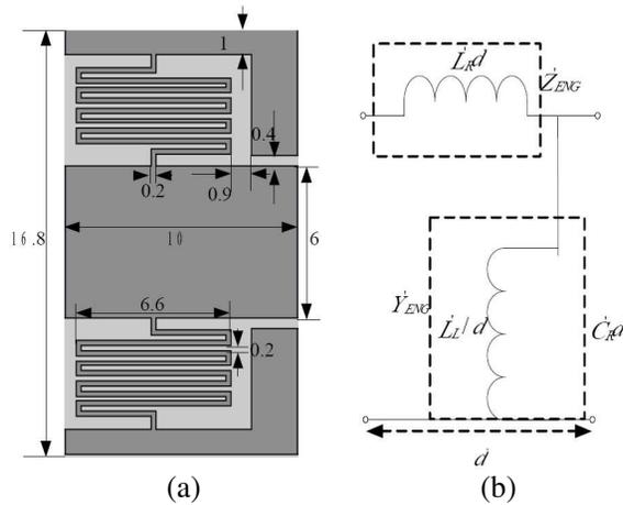
**Figure 1.** Structure of CPW ENG MTL (unit: mm). (a) Unit cell. (b) Equivalent circuit model.
