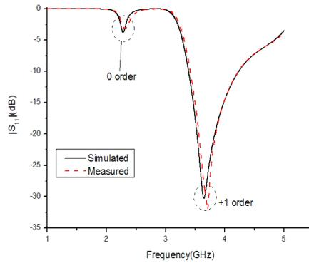
**Figure 6.** Simulated and measured return loss of the proposed CPW ENG MTL wideband antenna.
