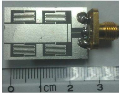
**Figure 5.** Fabricated wideband antenna.
