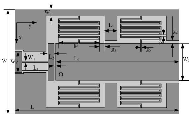
Figure 3. Configuration of the proposed CPW wideband antenna (unit: mm).
