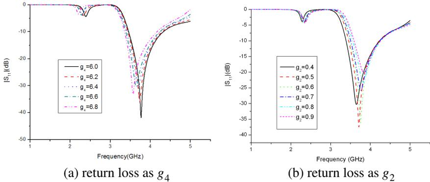
**Figure 4.** Return loss as parameters' change (Other parameters values are fixed).
