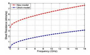
Figure 3. Comparison of sheet resistance versus frequency between new model and Ulrich's model.
