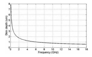
Figure 2. Skin depth of gold film VS frequency.
