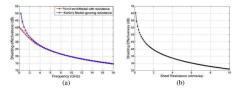
**Figure 6.** (a) Shielding effectiveness versus frequency and (b) sheet resistance.
