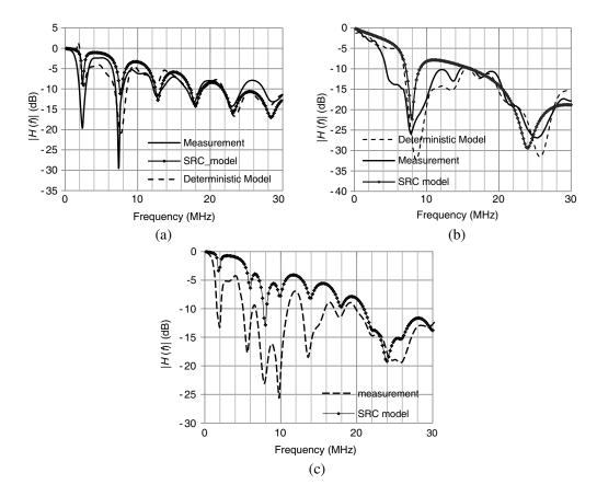
**Figure 10.** The measurements of (a) a single T-node, (b) the two T-node topology and (c) the three T-node topology compared to the SRC model analytical results.
