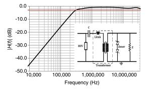
Figure 2. The coupler design and transfer function.
