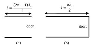
**Figure 9.** Types of transmission line series resonant circuits with length (a) a quarter wavelength and (b) a half wavelength.
