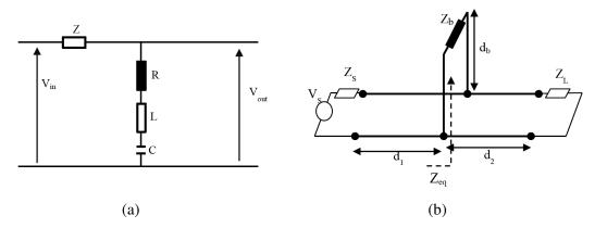
Figure 8. (a) The series resonant circuit. (b) The T-node topology connected to source and load.
