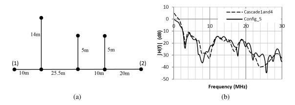
Figure 5. (a) The three T-node network. (b) Transfer function of the two networks cascade.
