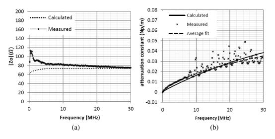
**Figure 1.** (a) The characteristic impedance for the  $2.5 \text{ mm}^2$  transmission line. (b) The measured and calculated attenuation coefficient for the  $2.5 \text{ mm}^2$  cable.
