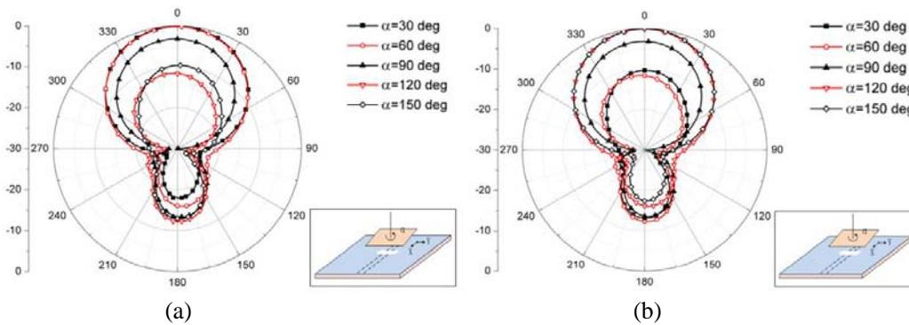
**Figure 2.** Simulated radiation patterns with different rotation angles of patches at 2.4 GHz: (a) LHCP at  $\phi = 0^\circ$ , (b) RHCP at  $\phi = 0^\circ$ .
