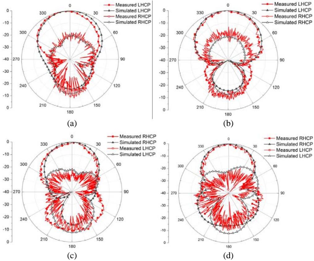
**Figure 9.** Simulated and measured normalized radiation patterns: (a) 2.18 GHz at  $xz$ -plane; (b) 2.18 GHz at  $yz$ -plane; (c) 2.87 GHz at  $xz$ -plane; (d) 2.87 GHz at  $yz$ -plane.
