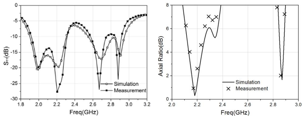
Figure 7. Measured reflection coefficient and AR of the proposed antenna.
