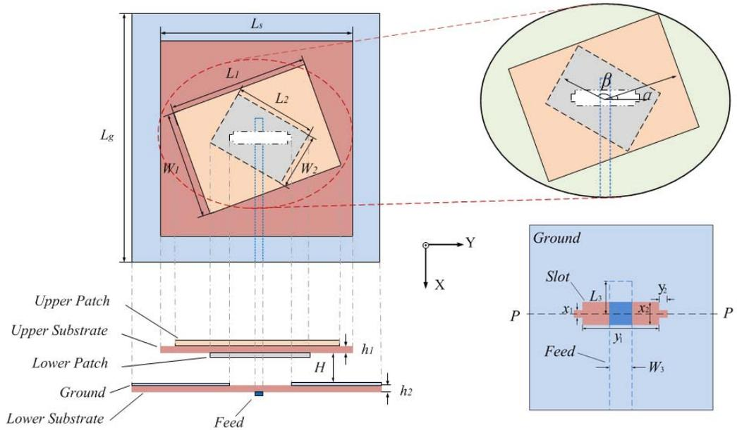
**Figure 1.** Schematic configuration of the proposed antenna.
