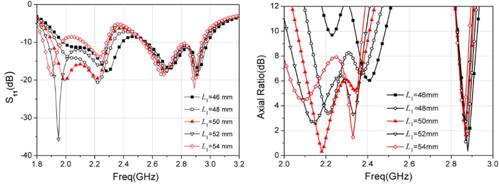
**Figure 4.** Simulated reflection coefficient and AR of proposed antenna with respect to various  $L_1$ .
