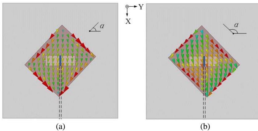
**Figure 3.** Surface current distributions on rotated patch at 2.4 GHz: (a)  $\alpha = 47^\circ$ , (b)  $\alpha = 134^\circ$ .
