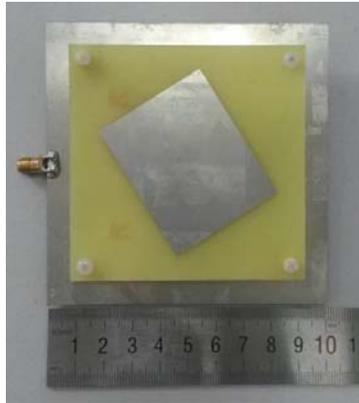
Figure 6. Photograph of the fabricated antenna.
