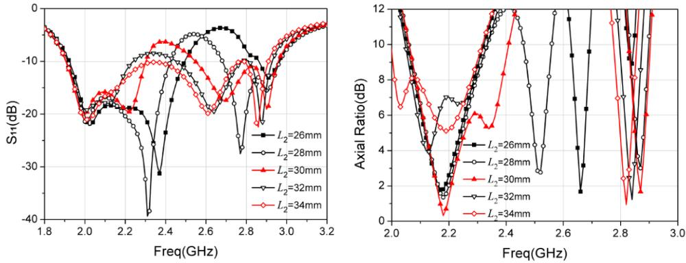
**Figure 5.** Simulated reflection coefficient and AR of proposed antenna with respect to various  $L_2$ .
