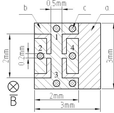
**Figure 1.** Geometry of galvanomagnetic transducer under research.
