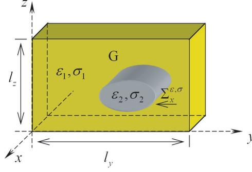
**Figure 1.** The cross section of one cells of the 2-D photonic crystal by two parallel planes  $x = \text{const}$ .
