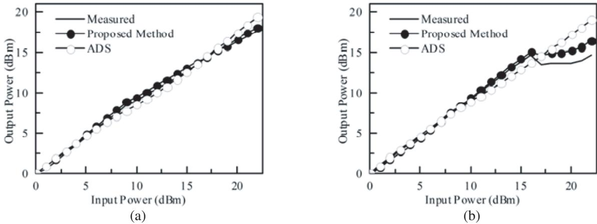
Figure 4. Output power vs. input power of the microstrip circuit for (a) 250 MHz and (b) 600 MHz.
