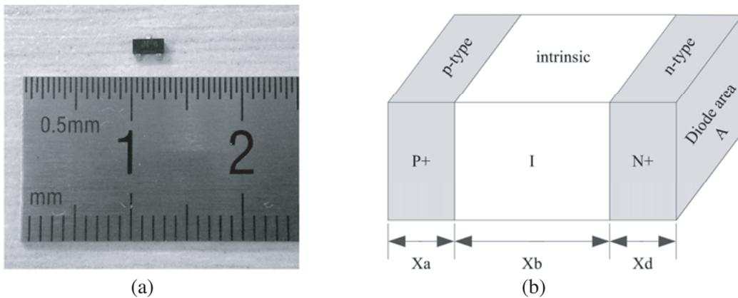
**Figure 2.** (a) A p-i-n diode with model number mot\_bal99lt1 and (b) its physical model.
