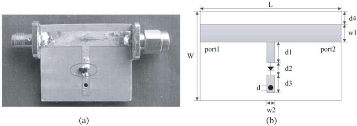
**Figure 3.** (a) Photo and (b) schematic plot of the microstrip diode circuit.
