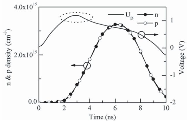
Figure 6. The simulated carrier densities at the center of i-layer during a forward voltage period.
