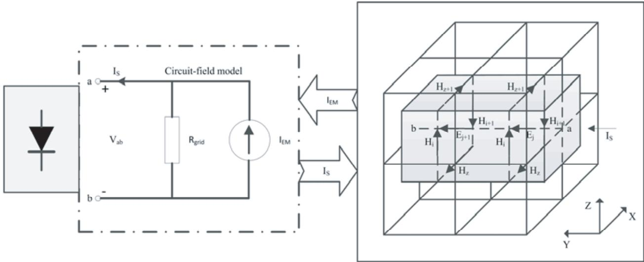
**Figure 1.** Illustration of the circuit-field model for coupling the external distributed structure with a diode.
