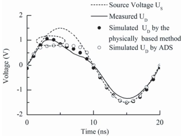
Figure 5. The measured and simulated terminal voltage waveforms of the chosen p-i-n diode.
