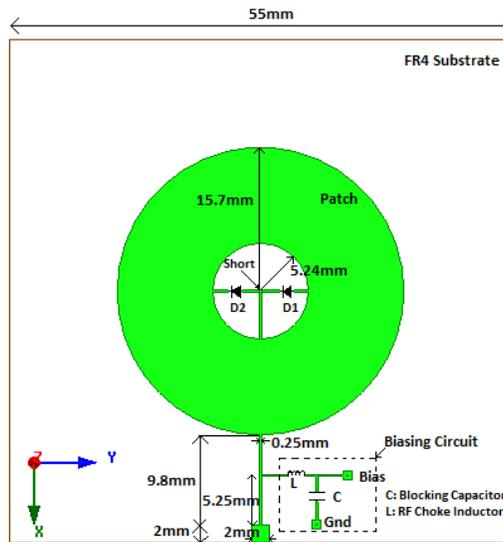
Figure 1. Antenna geometry.
