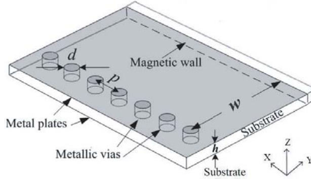
**Figure 1.** Structure of HMSIW.
