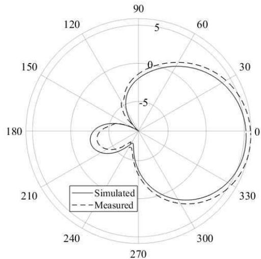
**Figure 6.** The  $E$ -plane radiation pattern of half-arrow slot antenna.
