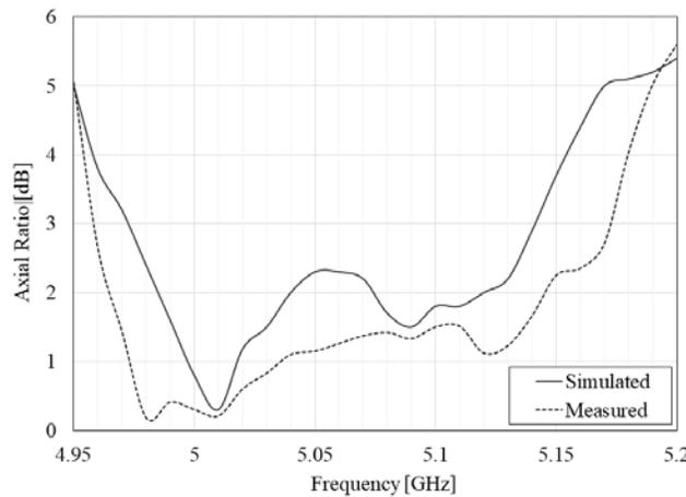
Figure 7. The axial ratio of half-arrow slot antenna.
