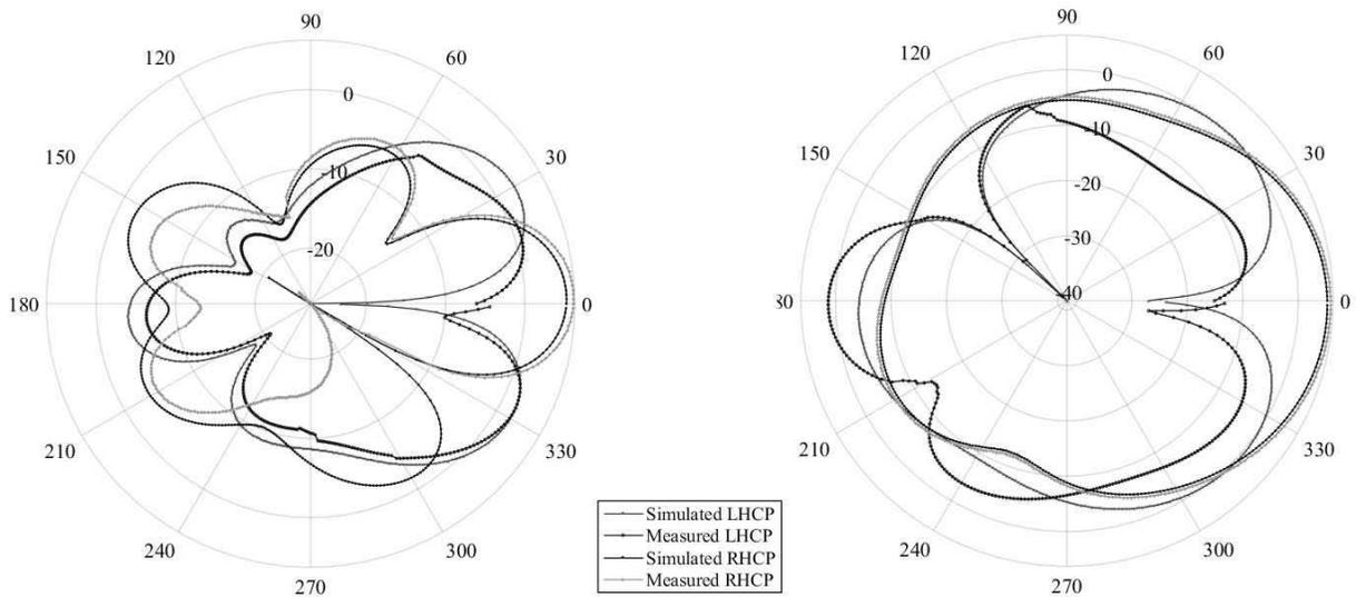
Figure 8. Simulated and measured radiation patterns in the  $XZ$ -plane ( $\varphi = 0^\circ$ ) and  $YZ$ -plane ( $\varphi = 90^\circ$ ).
