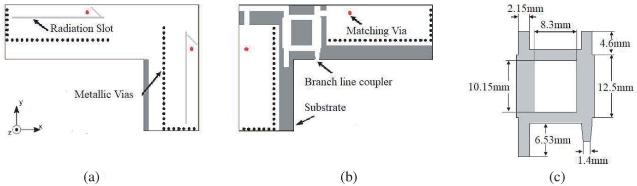
Figure 2. Configuration of CP antenna (a) front view and (b) back view, (c) coupler.
