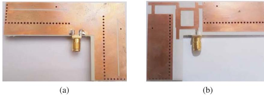
**Figure 4.** Fabricated two elements of HMSIW half-arrow slot antenna (a) front view and (b) back view.
