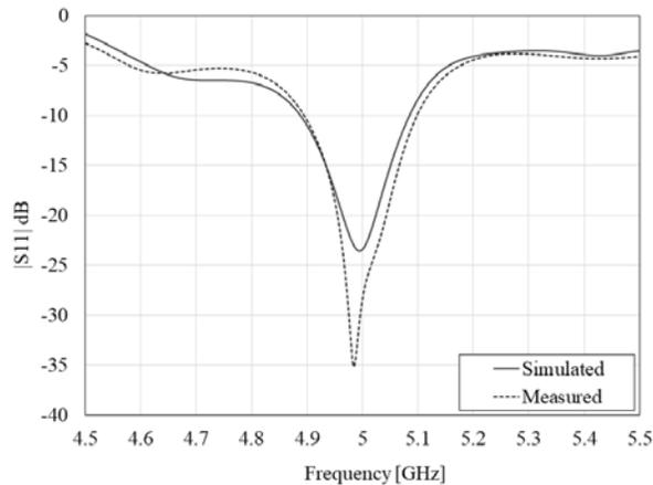
**Figure 5.** Measured versus simulated input return loss of the half-arrow slot antenna.
