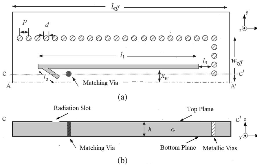
Figure 3. Layout of HMSIW half-arrow slot antenna element (a) top view and (b) side view along  $c-c'$ .
