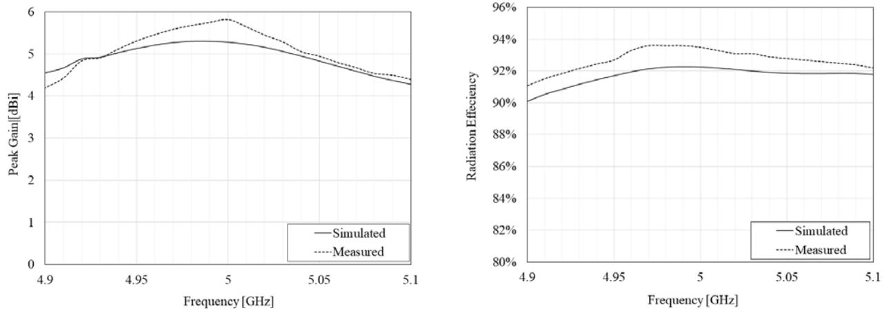
**Figure 9.** Gain and radiation-efficiency of the half-arrow antenna.
