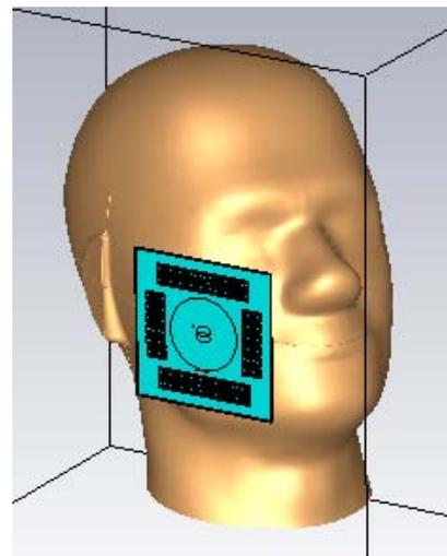
**Figure 5.** SAM phantom model and CMSA with EBG.
