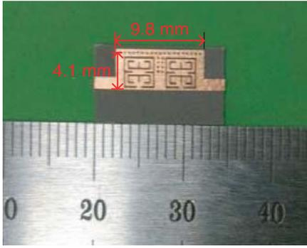
**Figure 9.** Photograph of the HMSIW-NSICSRR filter.
