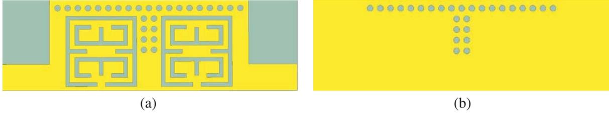
**Figure 8.** Structure diagram of the HMSIW-NSICSRR bandpass filter, (a) top view, (b) bottom view.
