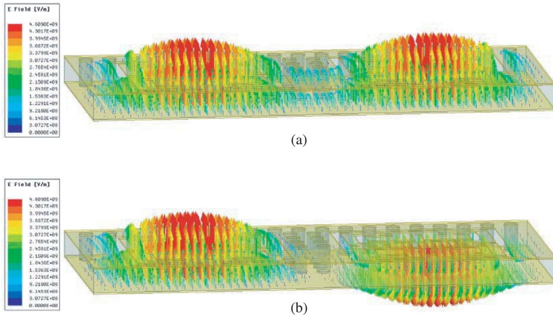
**Figure 5.** The resonant mode of the second order resonator with the dual-iris loading, (a) even mode, (b) the odd mode.
