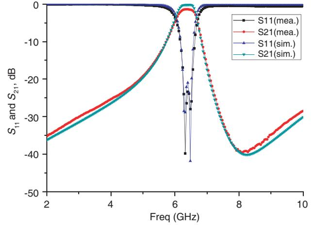
**Figure 10.** Simulated and measured  $S$ -parameters for HMSIW-NSICSRR filter.
