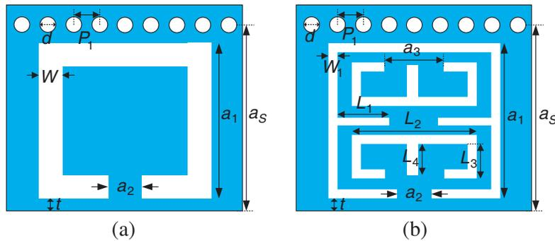
Figure 2. (a) Traditional HMSIW-CSRR resonant unit, (b) proposed HMSIW-NSICSRR resonant unit.
