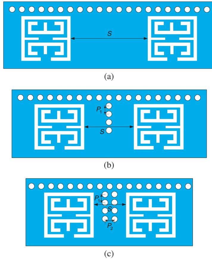
**Figure 4.** (a) Direct coupling scheme, (b) coupling scheme with single iris loading, (c) coupling scheme with dual-iris loading.
