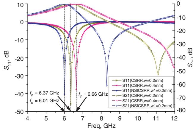
**Figure 3.** Simulated results comparison between traditional HMSIW-CSRR unit and proposed HMSIW-SICSRR unit.
