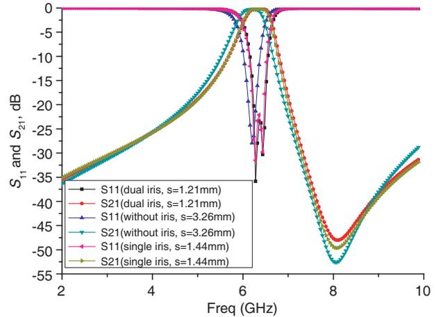
**Figure 7.** Simulated results of the HMSIW-NSICSRR bandpass filter with different kind of coupling schemes.
