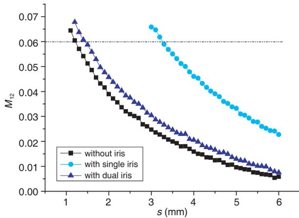
**Figure 6.** Simulated results comparison between coupling scheme with direct loading, single iris loading and dual-iris loading.
