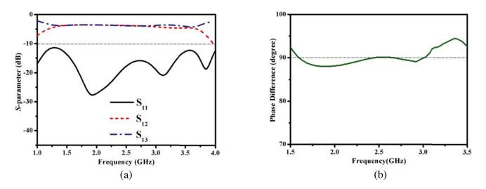
**Figure 4.** Simulated results of the designed broadband balun. (a) *S*-parameter; (b) phase difference of the two output ports.
