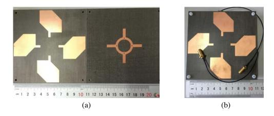
Figure 5. Prototype of the fabricated antenna. (a) Substrate 1 and substrate 2; (b) assembled antenna.
