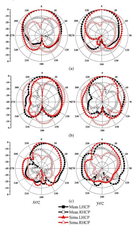
Figure 10. Simulated and measured radiation patterns of the proposed antenna in *xoz* and *yoz* planes. (a) 1.9 GHz; (b) 2.6 GHz and (c) 3.3 GHz for port 1.
