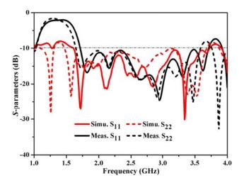
Figure 6. Simulated and measured S-parameters of the proposed antenna.
