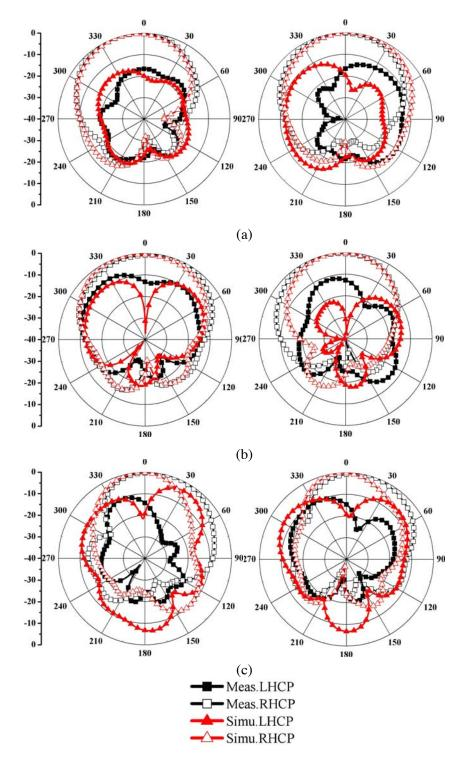
**Figure 11.** Simulated and measured radiation patterns of the proposed antenna in *xoz* and *yoz* planes. (a) 1.9 GHz; (b) 2.6 GHz and (c) 3.3 GHz for port 2.
