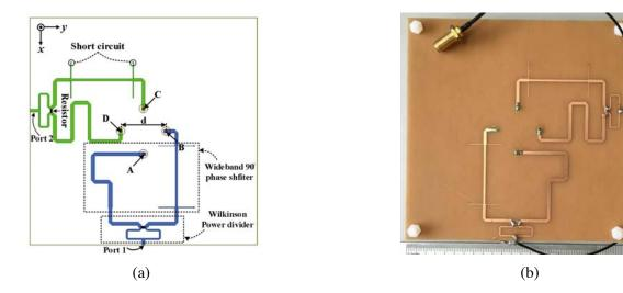
**Figure 3.** Configuration of broadband balun. (a) Layout graph of the balun; (b) photograph of the fabricated balun.
