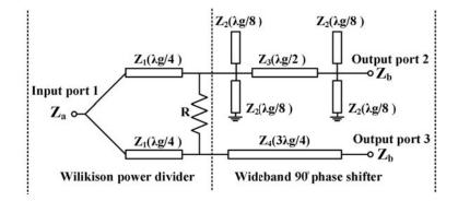
**Figure 2.** Circuit schematic of the microstrip balun.
