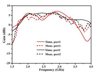
Figure 9. Simulated and measured gain of the proposed antenna in two ports.
