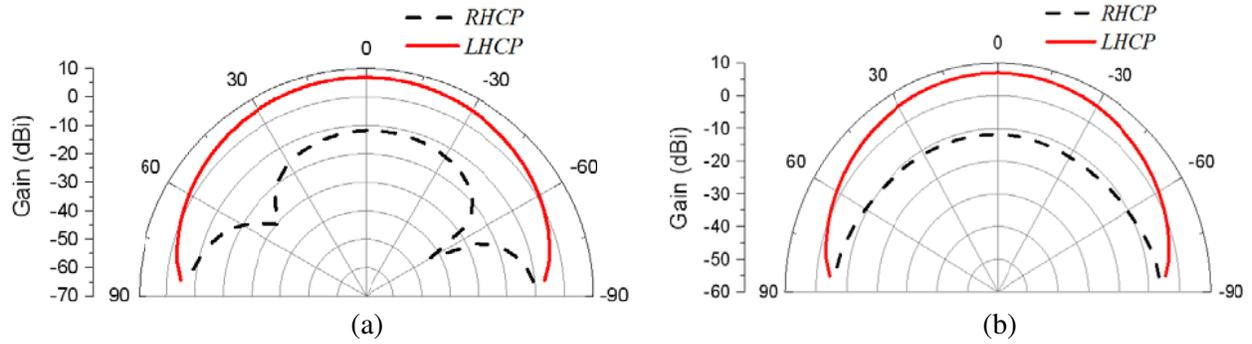
Figure 5. Radiation pattern at 2.45 GHz (a) *E*-plane (b) *H*-plane.
