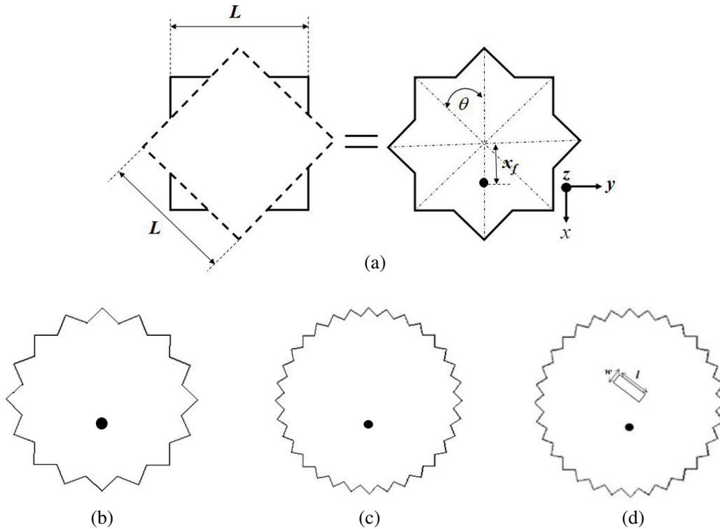
**Figure 1.** Antenna structure and geometrical evolution (a)  $45^\circ$  rotated square MPA (0th and 1st iteration), (b) SRFB MPA (2nd iteration), (c) SRFB MPA (3rd iteration), (d) Slotted SRFB with CP.
