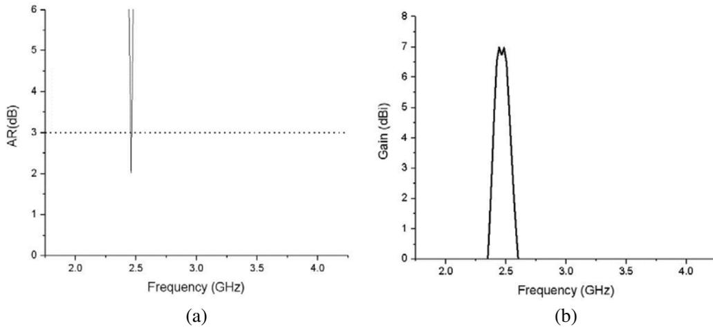
Figure 4. (a) Simulated axial ratio, (b) simulated gain characteristics.
