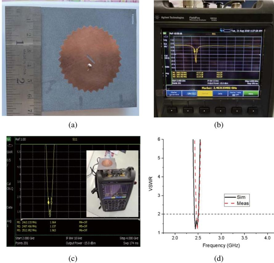
**Figure 7.** (a) Fabricated prototype. (b) Measured return loss. (c) Measured VSWR with experimental setup in inset. (d) Comparison between simulated and measured VSWR plot.
