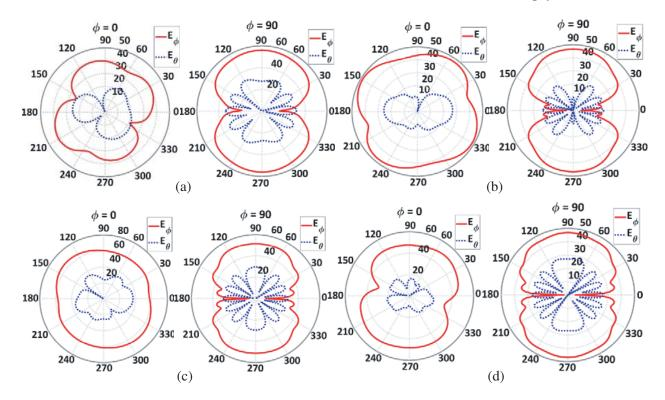
Figure 9. Radiation pattern of receive mode with  $Phi = 0^{\circ}$  and  $Phi = 90^{\circ}$  at (a) 8 GHz, (b) 9 GHz, (c) 10 GHz, (d) 11 GHz.
