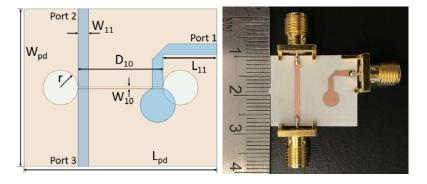
Figure 2. The top-view of the wideband power divider.
