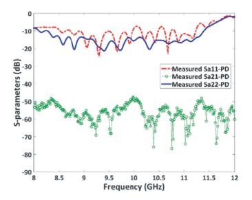
Figure 6. Measured S-parameters with power divider.
