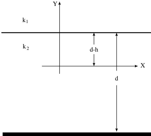
**Figure 2.** Geometry containing a grounded dielectric layer.
