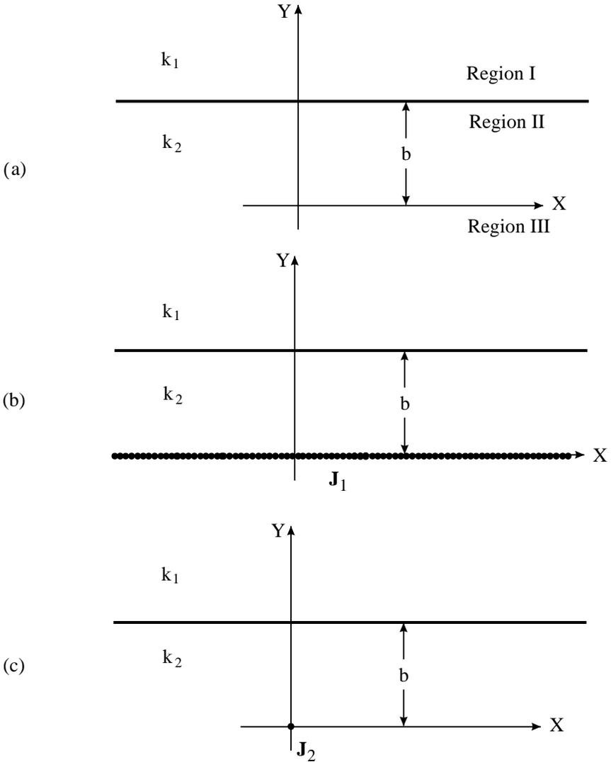
**Figure 1.** (a) Geometry containing a dielectric interface. (b) An infinite plate source is located at  $\delta(y)$  in a dielectric interface geometry. (c) An infinite line source is located at  $\delta(x)\delta(y)$  in a dielectric interface geometry.
