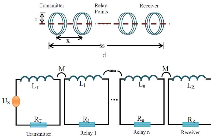
**Figure 4.** Magnetic waveguide and its circuit model.
