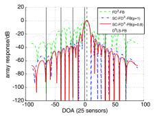
Figure 2. Beam pattern for  $SNR = 10 \, dB$  in 3° mismatch case.
