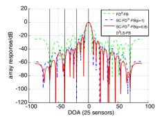
Figure 1. Beam pattern for  $SNR = 10 \, dB$  in no mismatch case.
