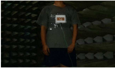
Figure 4. Antenna location on human chest.
