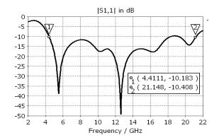
**Figure 9.** Simulated reflection coefficient of CPW antenna with optimal parameters.
