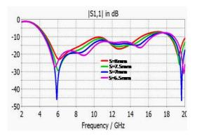
**Figure 6.** Simulated reflection coefficient curves for different *S* values.
