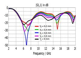
Figure 5. Simulated reflection coefficient curves for different  $Y_b$  values.
