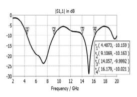
Figure 3. Simulated  $S_{11}$  reflection coefficient magnitude of the CPW antenna.
