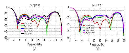
**Figure 7.** Simulated reflection coefficient curves for different (a)  $Y_a$  values and (b)  $X_a$  values.
