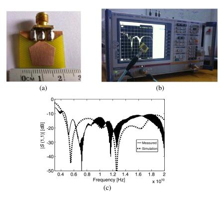
**Figure 11.** (a) Photograph of the fabricated antenna. (b) Bank under test. (c) Simulated and measured  $S_{11}$  parameter.
