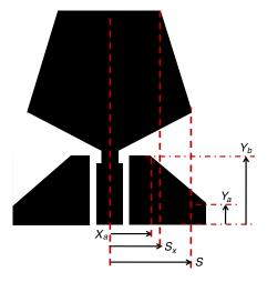
**Figure 4.** Geometry of the proposed CPW-fed pentagon antenna.
