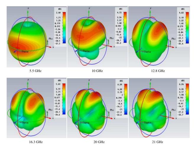
Figure 10. 3D plot of field pattern shows the gain at each selected frequency.
