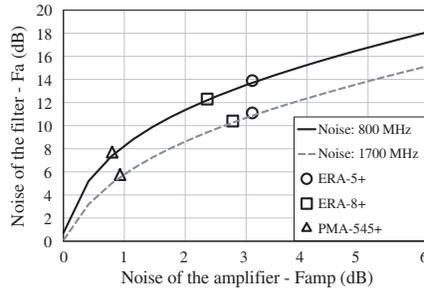
**Figure 13.** Simulated noise curves of the filter  $F_a$  as a function of the noise figure of the amplifier  $F_{amp}$  (from 9), and measured noise performance obtained with the ERA-5+, ERA-8+ and PMA-545+ amplifiers.
