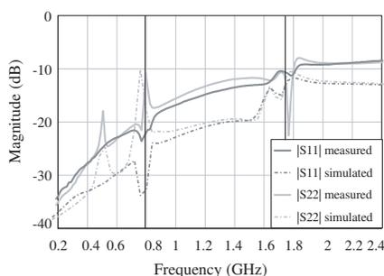
**Figure 16.** Reflection coefficients of the second-order active filter.
