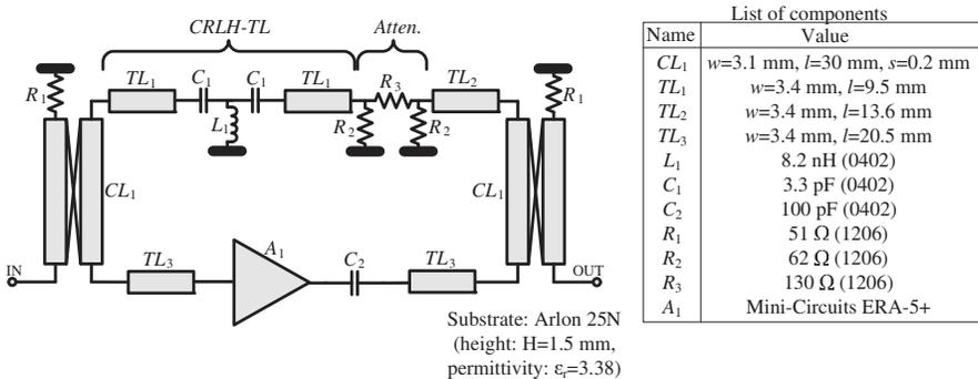
**Figure 8.** Circuit schematic and list of components of the first-order dual-band active filter prototype. The transmission lines are characterized by the width  $w$  and the length  $l$ . The coupled lines also include the separation gap  $s$ . The biasing network has been omitted for simplicity.
