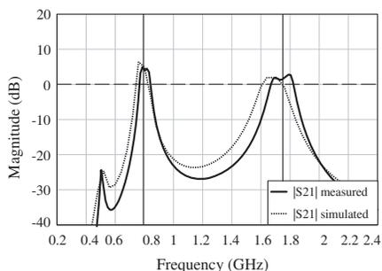
**Figure 15.** Transmission coefficient of the second-order active filter.
