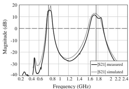
**Figure 18.** Transmission coefficient of the third-order active filter.
