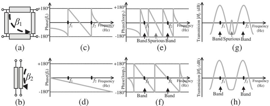
**Figure 7.** Comparison between feedback filters based on dual-band (top) or broadband (bottom) combiners: (a) (b) schematic of the power combiners, (c) (d) phase response of the combiners, (e) (f) phase response of the filter loop, and (g) (h) band-pass filter response.
