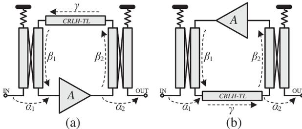
**Figure 4.** Two different active ring filter topologies.
