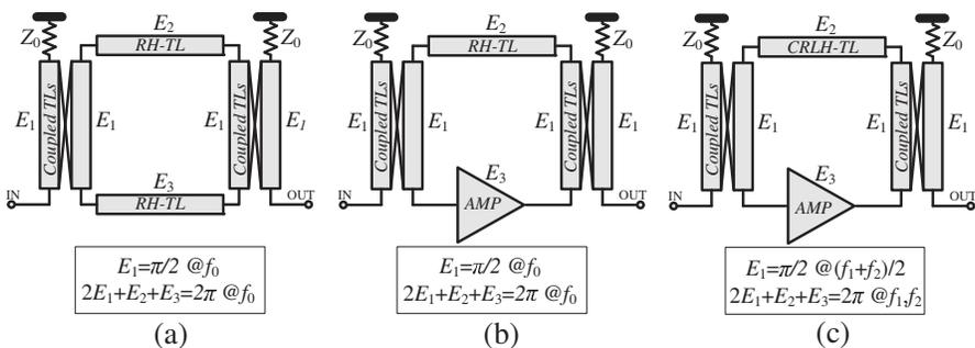
**Figure 3.** Ring resonator schemes: (a) Passive single-band, (b) active single-band and (c) proposed active dual-band topologies.  $E_i$  indicates the electrical length of each component, and  $Z_0$  is the reference impedance.
