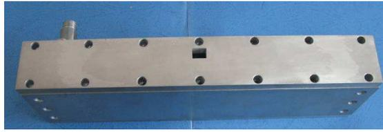
Figure 5. Photograph of the stripline resonator cavity.
