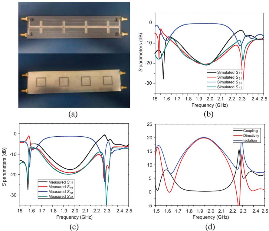
**Figure 7.** (a) Top (upper) and bottom (lower) sides of the fabricated coupler with parameters:  $R = 20$  mm,  $w = 1$  mm,  $g = 0.5$  mm,  $w_1 = 0.3$  mm,  $L_1 = 1.8$  mm,  $d = 0.2$  mm,  $L = 18$  mm,  $N = 21$ , the spacing between the two CRLH TLs is  $s = 1$  mm. (b) Full-wave simulated S parameters. (c) Measured S parameters, and (d) the three quantities characterizing the coupler.
