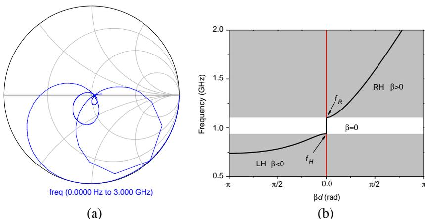
**Figure 2.** (a) Representation of the simulated reflection coefficient for the structures shown in Figure 1 on Smith Chart. (b) Simulated dispersion diagram obtained by Equation (8) with phase unwrapping.
