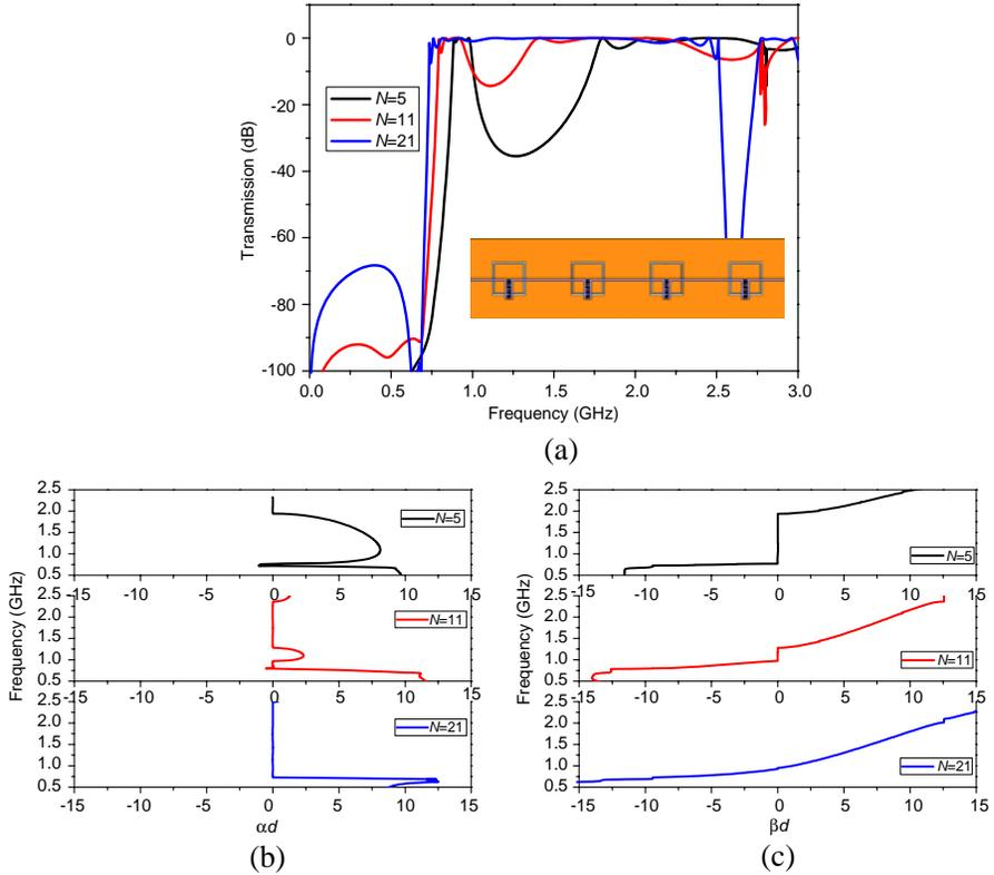
**Figure 4.** (a) Layout of the CRLH TL cascaded by four unit cells and the transmission response varies with the finger number  $N$  changing. (b) Attenuation, (c) dispersion diagrams computed by Equation (8) with phase unwrapping.
