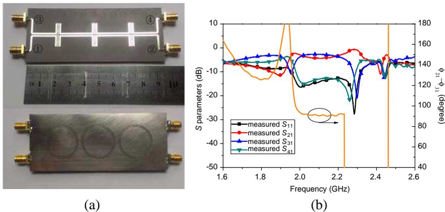
**Figure 8.** (a) Prototype of the 3-dB backward directional coupler constituted of two CRLH TLs with parameters:  $R = 12$  mm,  $w = 0.3$  mm,  $g = 0.3$  mm,  $w_1 = 0.2$  mm,  $L_1 = 1.8$  mm,  $d = 0.2$  mm,  $L = 11$  mm,  $N = 17$ , the spacing between the two CRLH lines is  $s = 0.5$  mm. (b) Measured results.
