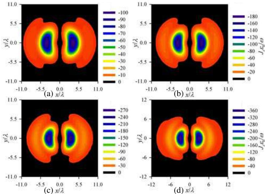
**Figure 3.** The orbital angular momentum density of the elegant Laguerre-Gaussian beam in the reference plane  $z = 20\lambda$ .  $w_0 = 5\lambda$  and  $m = 2$ . (a)  $n = 2$ . (b)  $n = 3$ . (c)  $n = 4$ . (d)  $n = 5$ .
