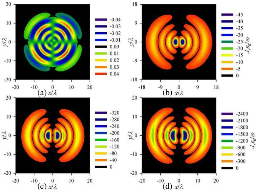
**Figure 5.** The orbital angular momentum density of the standard Laguerre-Gaussian beam in the reference plane  $z = 20\lambda$ .  $w_0 = 5\lambda$  and  $n = 3$ . (a)  $m = 0$ . (b)  $m = 1$ . (c)  $m = 2$ . (d)  $m = 3$ .
