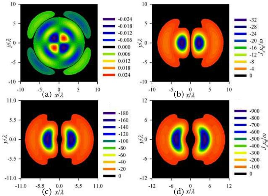
**Figure 2.** The orbital angular momentum density of the elegant Laguerre-Gaussian beam in the reference plane  $z = 20\lambda$ .  $w_0 = 5\lambda$  and  $n = 3$ . (a)  $m = 0$ . (b)  $m = 1$ . (c)  $m = 2$ . (d)  $m = 3$ .
