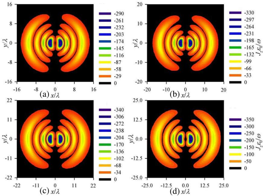
**Figure 7.** The orbital angular momentum density of the standard Laguerre-Gaussian beam in the reference plane  $z = 20\lambda$ .  $m = 2$  and  $n = 3$ . (a)  $w_0 = 4\lambda$ . (b)  $w_0 = 5\lambda$ . (c)  $w_0 = 6\lambda$ . (d)  $w_0 = 7\lambda$ .
