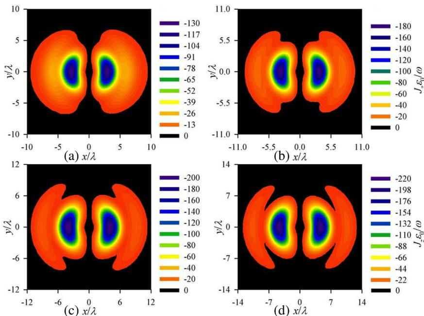
**Figure 4.** The orbital angular momentum density of the elegant Laguerre-Gaussian beam in the reference plane  $z = 20\lambda$ .  $m = 2$  and  $n = 3$ . (a)  $w_0 = 4\lambda$ . (b)  $w_0 = 5\lambda$ . (c)  $w_0 = 6\lambda$ . (d)  $w_0 = 7\lambda$ .
