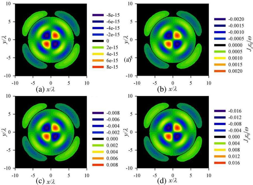
**Figure 1.** The orbital angular momentum density of the elegant Laguerre-Gaussian beam in different reference planes.  $w_0 = 5\lambda$ ,  $n = 3$ , and  $m = 0$ . (a)  $z = 0$ . (b)  $z = 5\lambda$ . (c)  $z = 10\lambda$ . (d)  $z = 15\lambda$ .
