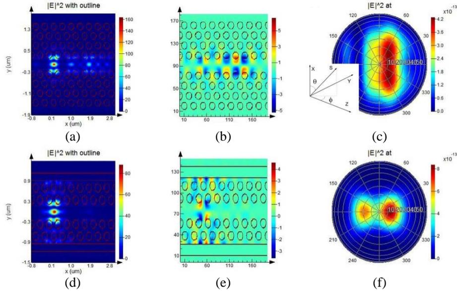
**Figure 4.** (a) & (d) Time-averaged power distribution of  $|E|^2$  in normal and HPhC waveguides, respectively. (b) & (e) The corresponding electric field  $E_y$ . (c) & (f) The corresponding far-field pattern obtained at the observation plane.
