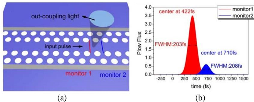
**Figure 3.** (a) Structure for exciting pulse and schematic diagram for interrogation. (b) The waveform is captured by the line monitor, with amplitude 1 at  $0.227 \mu\text{m}$ , 60 fs and amplitude 0.19 at  $1.465 \mu\text{m}$ , 829 fs. The working point is chosen at  $(k_x, f) = (0.1, 0.299984c/\Lambda)$ .
