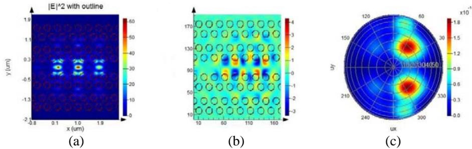
**Figure 6.** (a) Time-averaged power distribution of  $|E|^2$  in normal waveguide with lateral shift  $\Delta = 150$  nm. (b) The corresponding electric field  $E_y$ . (c) The corresponding far-field pattern calculated at the observation plane.
