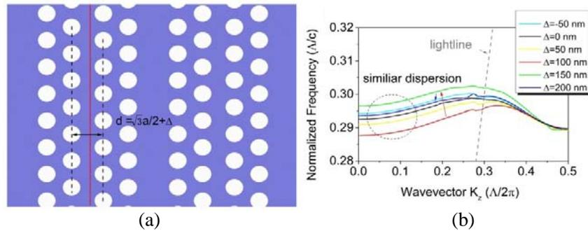
**Figure 5.** (a) Schematic diagram of the normal PhC waveguide with partial lateral shift  $\Delta$ . The lateral shift occurs at the gap between the first and the second row of air hole. (b) The corresponding dispersion for PhC waveguides with different  $\Delta$ . All the sweep parameters are labeled in the legend. The rising and falling behaviors are depicted by the red and blue arrows, respectively. The turning point for the dispersion is at  $\Delta = 150$  nm.
