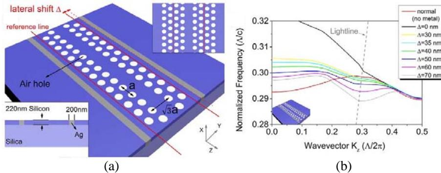
**Figure 1.** (a) Schematic of the proposed HPhC waveguide. The cross section of the structure is shown in the lower left inset. (b) Dispersion curves for the HPhC waveguides with varying lateral shift  $\Delta$ .
