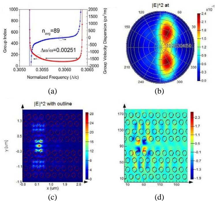
**Figure 8.** (a) Average group index and GVD for  $\Delta = 100$  nm. (b) The corresponding far-field pattern calculated at the observation plane. The working point is chosen at  $(k_x, f) = (0.1, 0.3062510c/\Lambda)$ . (c) Time-averaged power distribution of  $|E|^2$  in normal and HPhC waveguide. (d) The corresponding component  $E_y$  of electric field.
