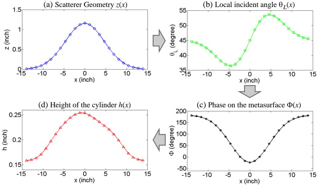
**Figure 3.** Graded metasurface design flowchart (a) Scatterer geometry vs. position  $x$ . (b) Local incident angle vs. position  $x$ . (c) Phase shift vs. position  $x$ . (d) Height of the cylinder vs. position  $x$ .
