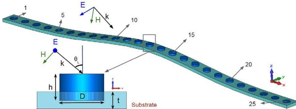
**Figure 2.** Schematic of the entire metasurface, discretized with 25 cylinders, and coordinate system. (Inset) unit cell of the metasurface. The bottom black line is the ground plane, the light blue substrate is Teflon, and the dark blue cylinder is ceramic. The incident wave is polarized along the  $y$  axis.
