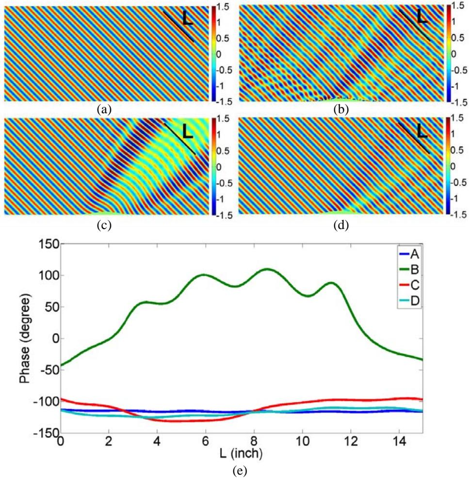
**Figure 5.** (a) Electric field reflection pattern for a flat ground plane. (b) Electric reflection pattern for a Gaussian scatterer with dielectric cylinders cloaking metasurface. (c) Electric field reflection pattern for a Gaussian scatterer. (d) Electric field reflection pattern for a Gaussian scatterer with more continuously varying refractive index. (E) Phase plot along the equi-phase line  $L$  in (a)–(d).
