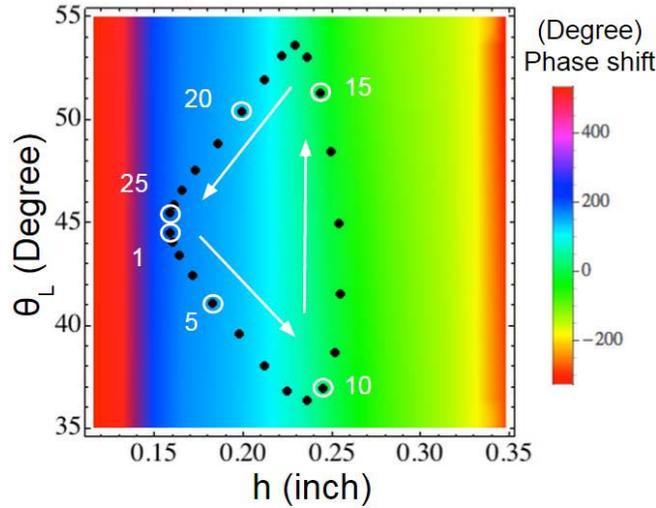
**Figure 4.** Simulated phase shift with varying height  $h$  and local incident angle  $\theta_L$  for a frequency of 4.15 GHz. The dark points correspond to the different heights chosen for the 25 cylinders on the metasurface.
