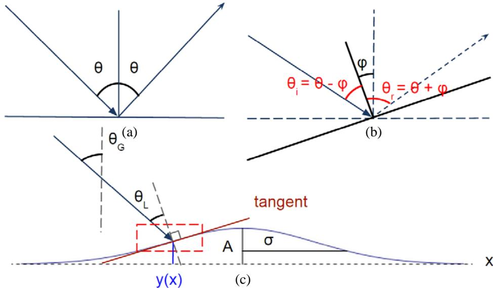
**Figure 1.** (a) Reflection from a flat plane. (b) Reflection from a flat plane with a counterclockwise rotation by an angle  $\varphi$ . Cases A and B are both governed by Snell's law. (c) Reflection from a Gaussian scatterer that can be treated locally, at each point along the surface, as a flat plane.
