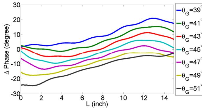
**Figure 6.** Phase difference on the equi-phase line  $L$  between the phase reflected by our metasurface (designed for 45 degree) and phase expected from a flat ground plane for different global incident angles.
