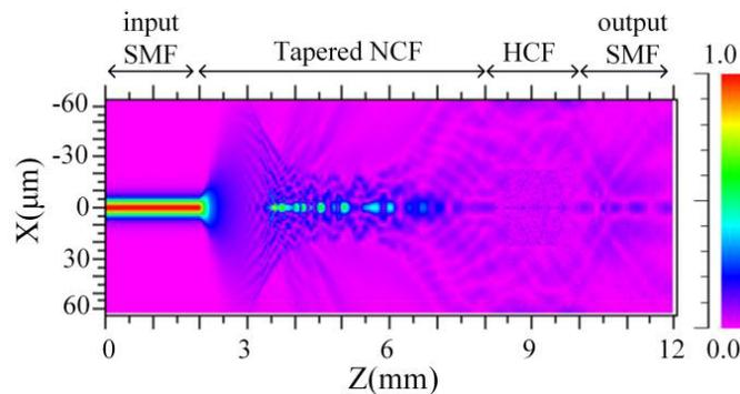
**Figure 4.** Simulated optical field intensity distribution within the TNHF ( $L_1 = 6$  mm,  $D = 37$   $\mu$ m).
