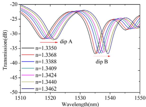
Figure 6. Transmission spectrum evolution when SRI is changed.
