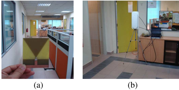
Figure 9. Measurement setup (a) receiver (RFID tag), (b) transmitter (RFID reader).
