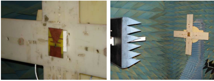
Figure 6. Measurement of proposed multi-band antenna's radiation pattern.
