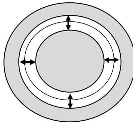
**Figure 1.** Stator deformations for  $m = 0$ .
