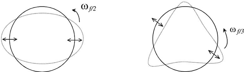
**Figure 2.** Stator deformations for  $m = 2$  and 3.
