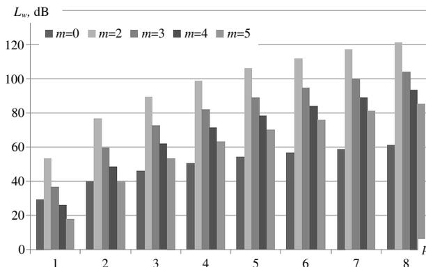
**Figure 8.** Variation of the acoustic power level (due to magnetic phenomena) with  $p$  and  $f$ .
