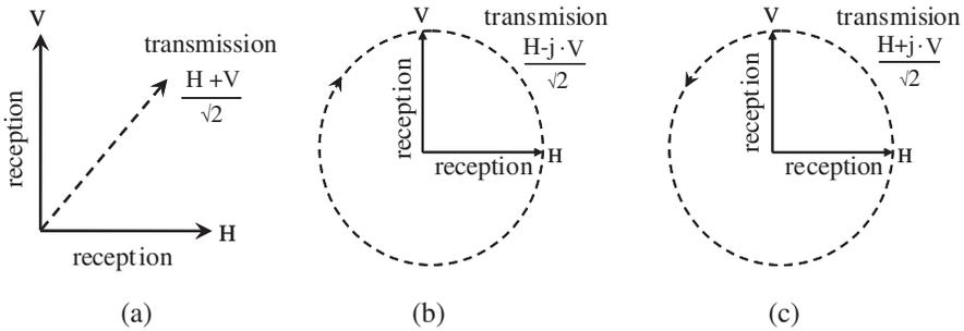
**Figure 1.** Schematic diagrams showing different hybrid polarimetric imaging modes where the transmission polarization is shown in dotted lines and reception polarizations are shown in solid lines. (a)  $\pi/4$  mode. (b) Right circular hybrid mode. (c) Left circular hybrid mode.
