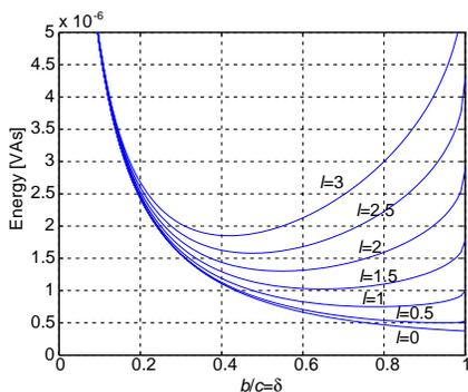
**Figure 3.** Plot of the energy for different combinations of currents for a varying number turns  $l$  as a function of  $c/b$  when  $m = 1$  and  $bc = 1$ .
