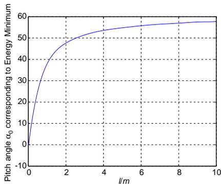
**Figure 4.** Pitch angle  $\alpha_0$  for a torus as a function of the ratio  $l/m$ . The angle approaches  $90^\circ$  monotonically, but very slowly.
