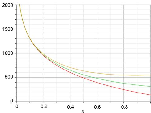
**Figure 8.** Plot of the functions  $f_\gamma$  of Eq. (65) giving the inductance for current densities  $\sim \rho^\gamma$  in a thin ring. The top curve corresponds to  $\gamma = 1$ , the middle one to  $\gamma = 0$ , and the bottom curve to  $\gamma = -1$ . Note that the  $\gamma$ -ordering here is the same as in Fig. 6 for surface currents.
