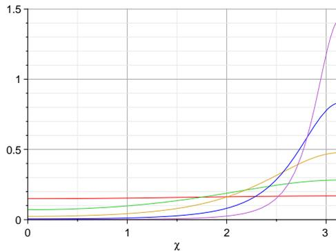
**Figure 7.** The normalised current density  $J_\varphi(\chi) = j_\varphi(\psi(\chi))$  on the superconducting torus as a function of  $\chi$  which is zero on the outside of the torus and  $\pi$  on the inside. The current peaks on the inside. The values of  $\xi$  shown are  $c/b = \xi = 1.1, 1.3, 2.0, 5.0, 100$ , the slowly varying curves corresponding to the larger  $\xi$ .
