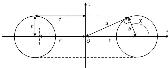
**Figure 1.** Section of torus in the  $xz$ -plane. The major radius is denoted  $c$ , the minor radius  $b$ . The length parameter  $a$  of the toroidal coordinates then obeys,  $a^2 + b^2 = c^2$ , as illustrated by the right angled triangle.
