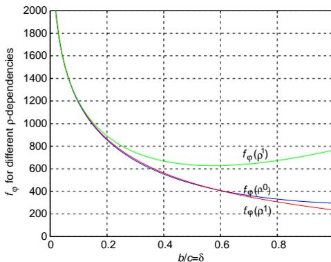
**Figure 6.** Plot of the functions  $f_\varphi$  giving the inductance for various surface current densities on a torus. Note that the curve  $f_\varphi(\rho^0)$  is the same as the upper curve in Fig. 5.
